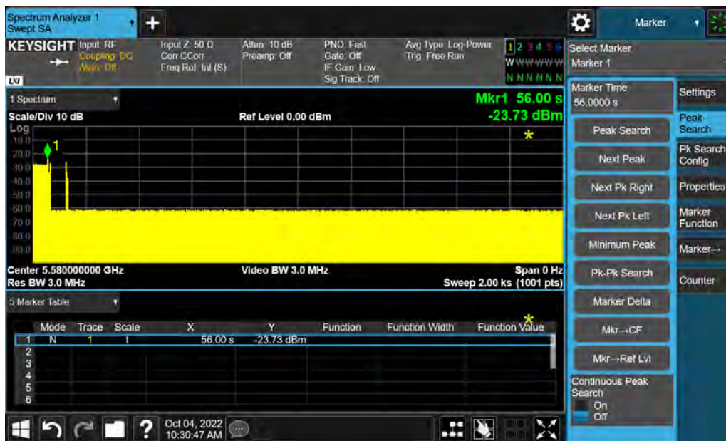
Plot 10: Client Radar Injection- Client Non-Occupancy
