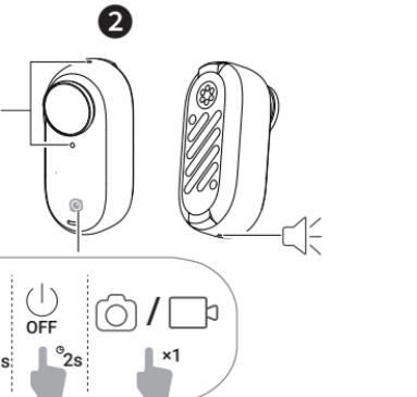
Press for 3 seconds to power on, press for 2 seconds to power off, and press once to start taking photos or recording videos.
