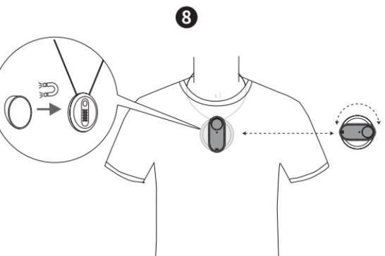
First, attach the spacer to the Magnet Pendant and put it into your clothes. Then attach GO 3 to the Magnet Pendant.
