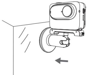
Remove the pad cover from the bottom and paste the Pivot Stand with GO 3 to a smooth, clean surface.
