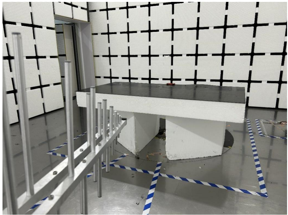
Radiation Emission Test Setup (30MHz to 1GHz)
