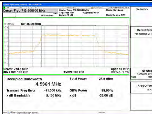
Band17 / 5MHz / 64QAM/ High CH
