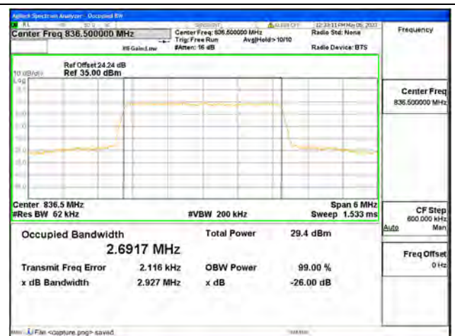
Band5 / 3MHz / 16QAM/ Mid CH
