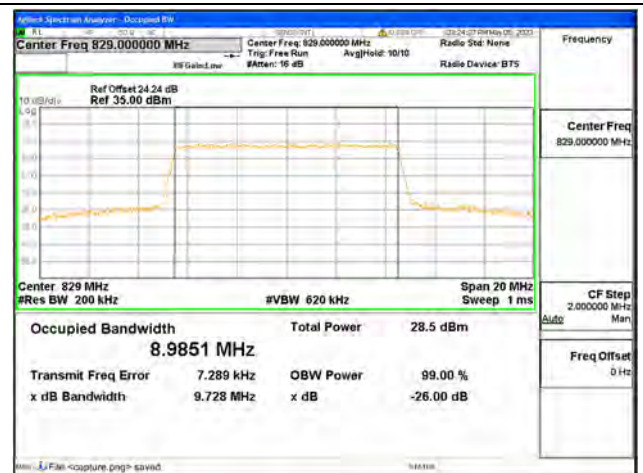
Band5 / 10MHz / 64QAM/ Low CH
