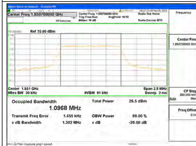
Band2 / 1.4MHz / 64QAM/ Low CH
