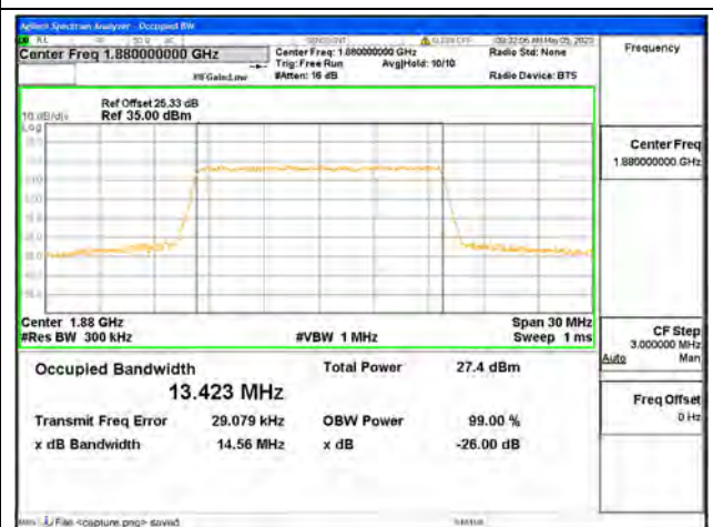
Band2 / 15MHz / 64QAM/ Mid CH
