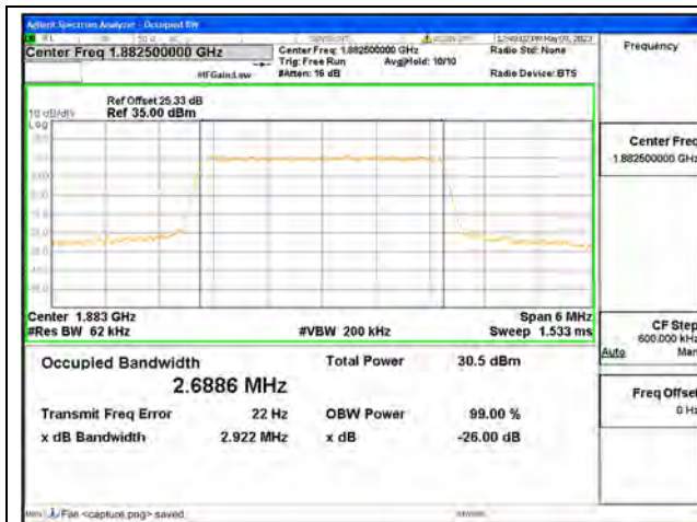
Band25 / 3MHz / QPSK/ Mid CH
