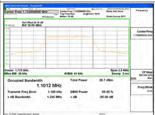
Band4 / 1.4MHz / 64QAM/ Mid CH
