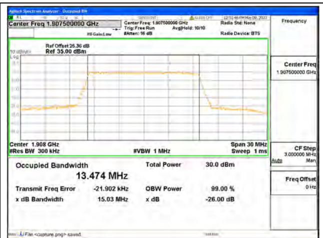
Band25 / 15MHz / 16QAM/ High CH
