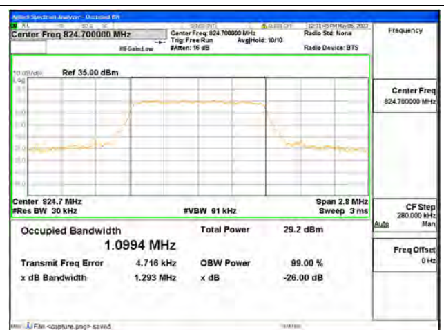
Band5 / 1.4MHz / 16QAM/ Low CH
