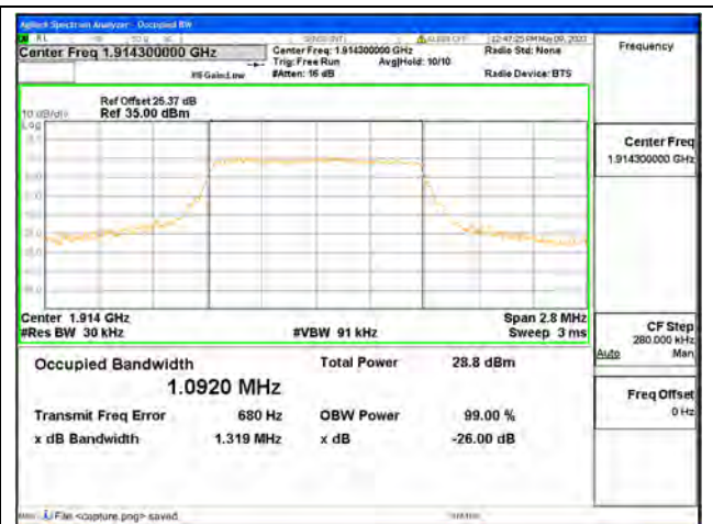
Band25 / 1.4MHz / 16QAM/ High CH
