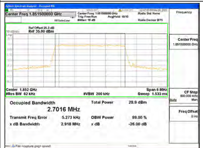
Band25 / 3MHz / 64QAM/ Low CH
