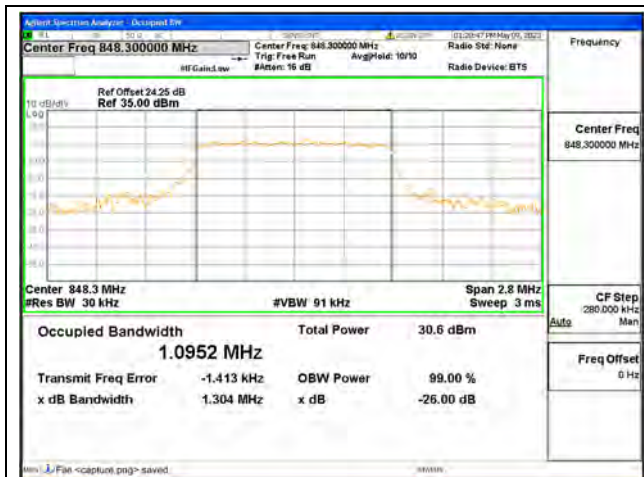
Band26 Part22 / 1.4MHz / QPSK/ High CH
