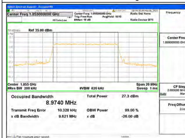
Band2 / 10MHz / 16QAM/ Low CH
