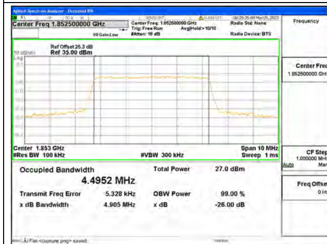
Band2 / 5MHz / 64QAM/ Low CH
