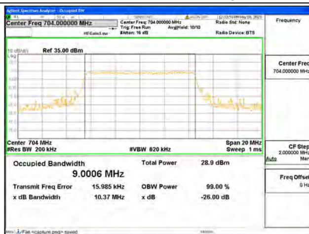
Band12 / 10MHz / 16QAM/ Low CH
