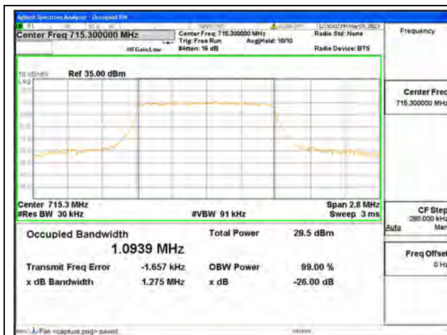
Band12 / 1.4MHz / QPSK/ High CH
