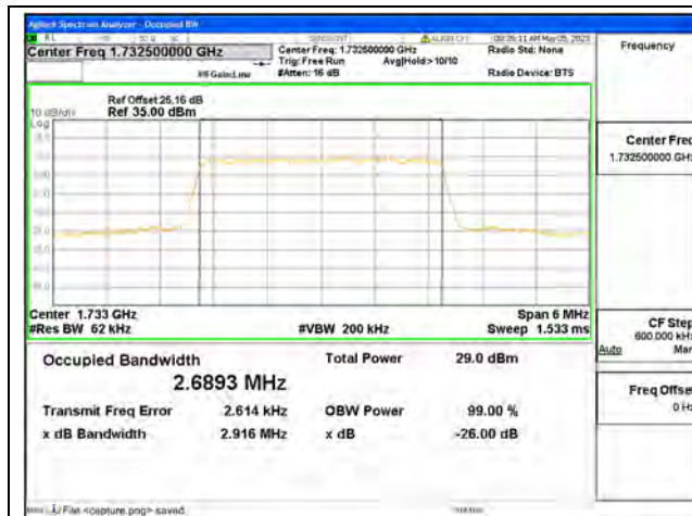
Band4 / 3MHz / QPSK/ Mid CH
