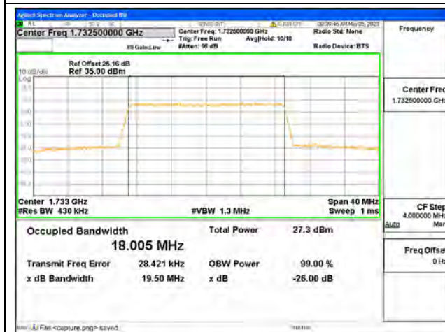
Band4 / 20MHz / 64QAM/ Mid CH
