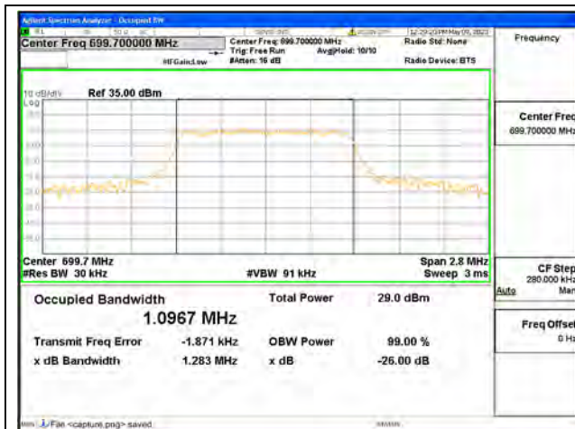
Band12 / 1.4MHz / QPSK/ Low CH
