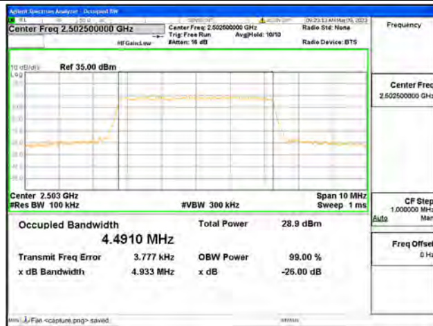
Band7 / 5MHz / 64QAM/ Low CH
