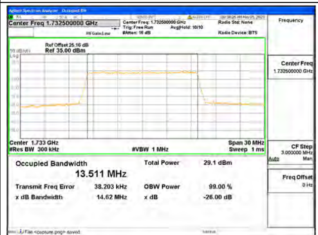
Band4 / 15MHz / QPSK/ Mid CH
