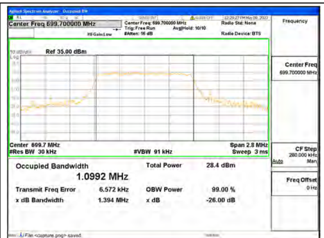
Band12 / 1.4MHz / 16QAM/ Low CH
