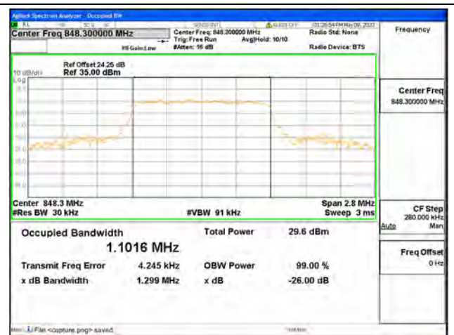
Band26 Part22 / 1.4MHz / 16QAM/ High CH
