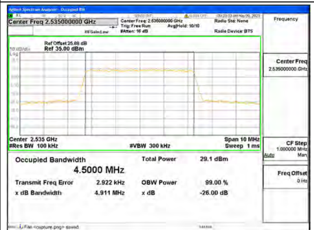
Band7 / 5MHz / 64QAM/ Mid CH
