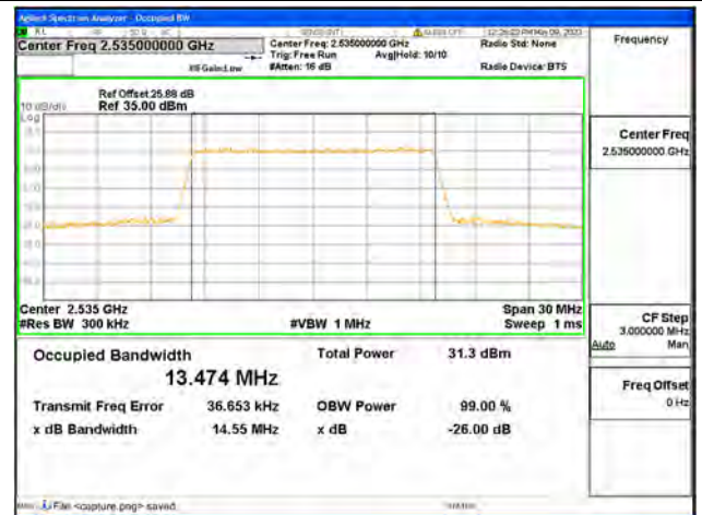
Band7 / 15MHz / QPSK/ Mid CH
