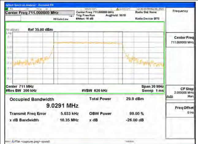
Band17 / 10MHz / QPSK/ High CH
