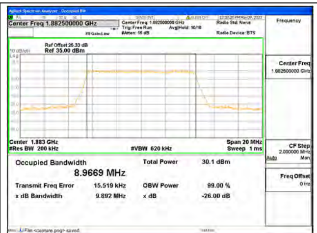
Band25 / 10MHz / 16QAM/ Mid CH
