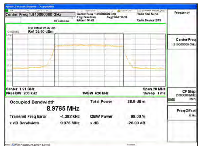
Band25 / 10MHz / 64QAM/ High CH
