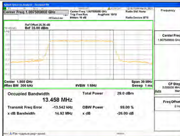
Band25 / 15MHz / 64QAM/ High CH
