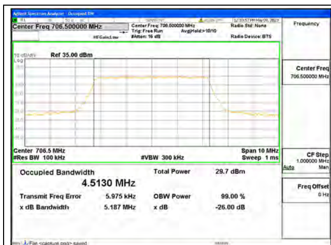
Band17 / 5MHz / QPSK/ Low CH
