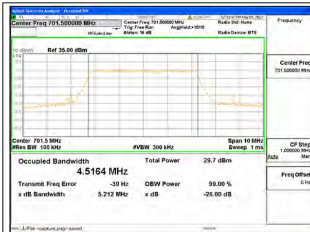
Band12 / 5MHz / QPSK/ Low CH
