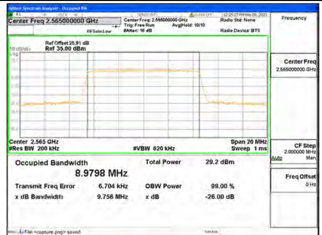
Band7 / 10MHz / 64QAM/ High CH
