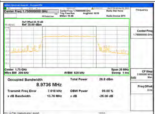
Band4 / 10MHz / 64QAM/ High CH
