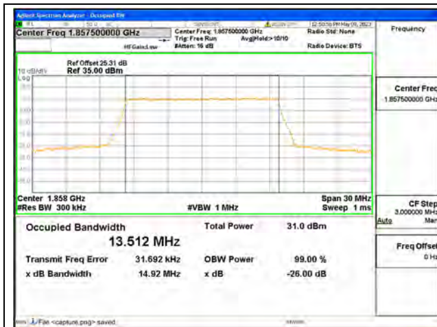
Band25 / 15MHz / QPSK/ Low CH
