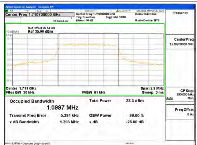
Band4 / 1.4MHz / 16QAM/ Low CH
