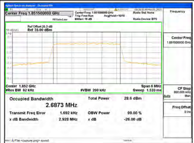
Band2 / 3MHz / QPSK/ Low CH
