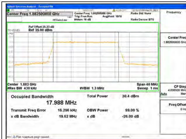
Band25 / 20MHz / QPSK/ Mid CH
