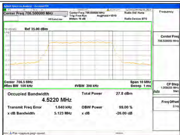
Band17 / 5MHz / 64QAM/ Low CH
