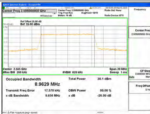
Band7 / 10MHz / 16QAM/ Low CH
