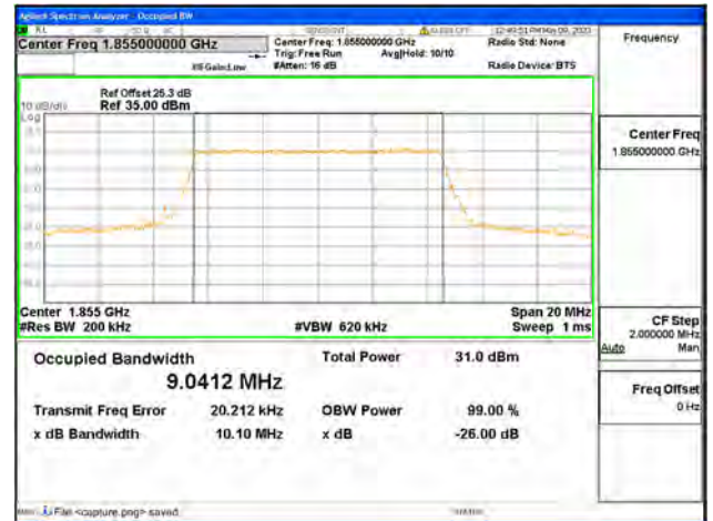
Band25 / 10MHz / QPSK/ Low CH
