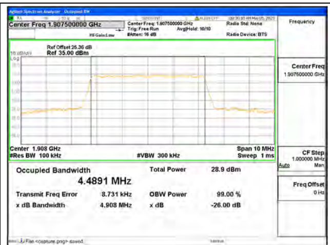
Band2 / 5MHz / 16QAM/ High CH
