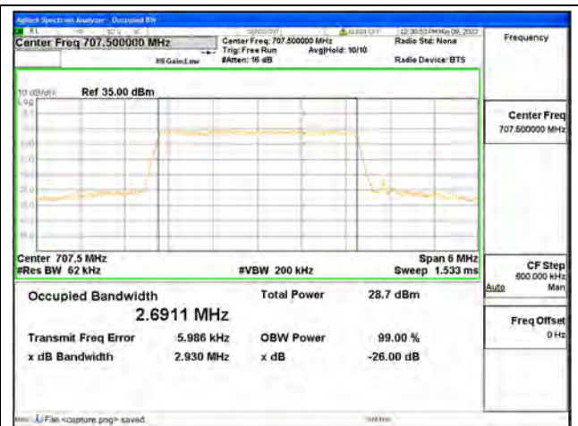
Band12 / 3MHz / 16QAM/ Mid CH
