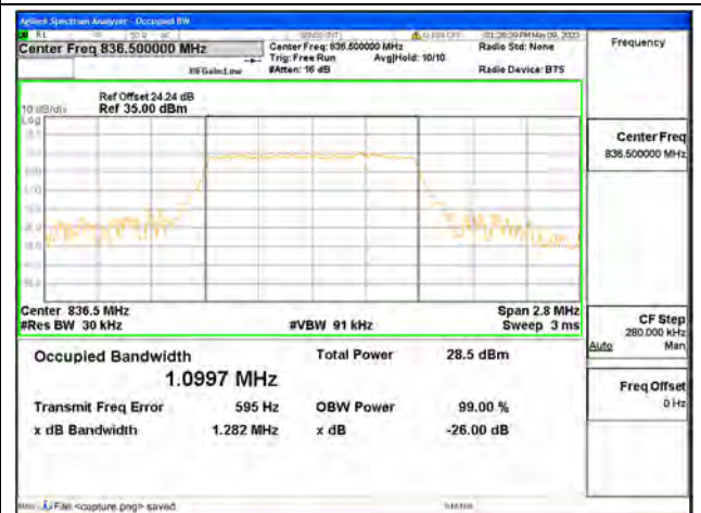
Band26 Part22 / 1.4MHz / 64QAM/ Mid CH
