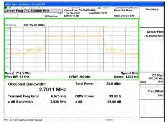
Band12 / 3MHz / QPSK/ High CH
