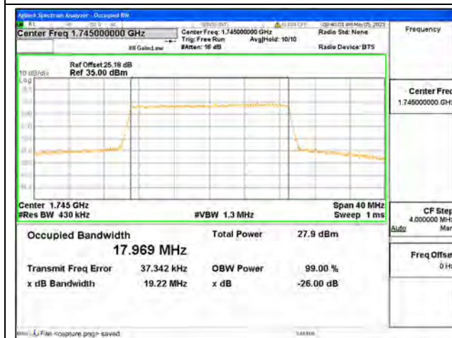
Band4 / 20MHz / 16QAM/ High CH
