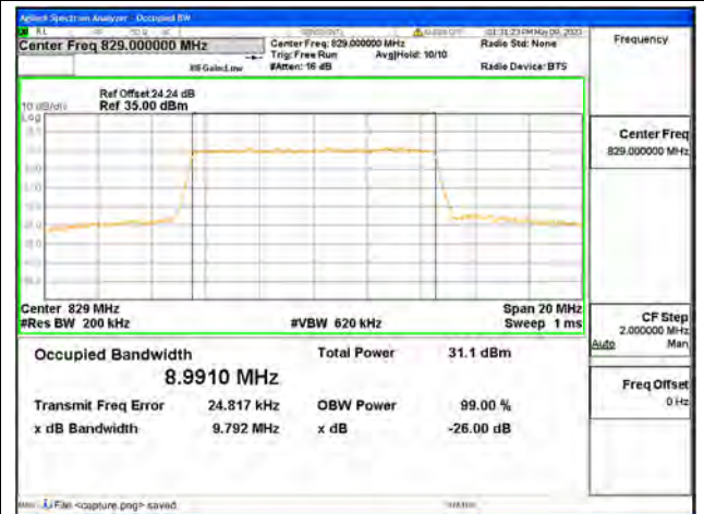
Band26 Part22 / 10MHz / QPSK/ Low CH
