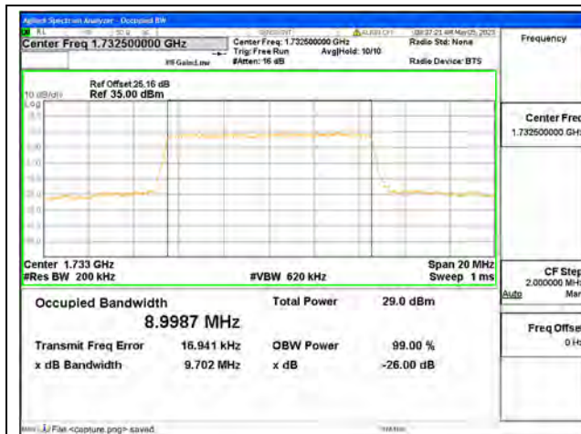
Band4 / 10MHz / QPSK/ Mid CH
