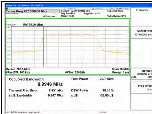
Band12 / 10MHz / QPSK/ Mid CH
