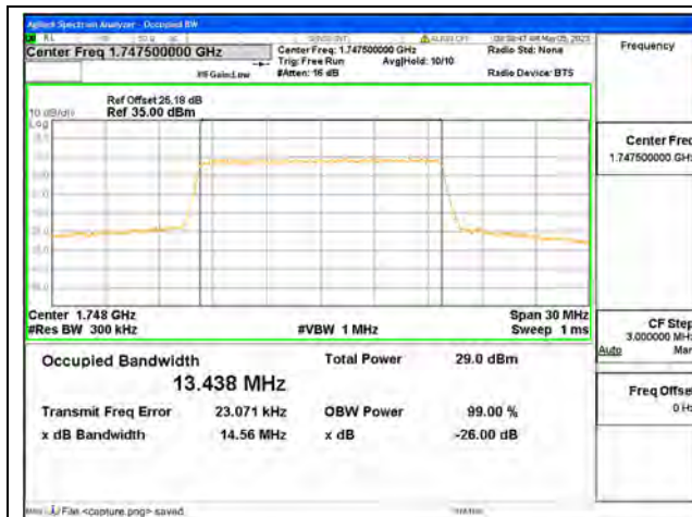
Band4 / 15MHz / QPSK/ High CH
