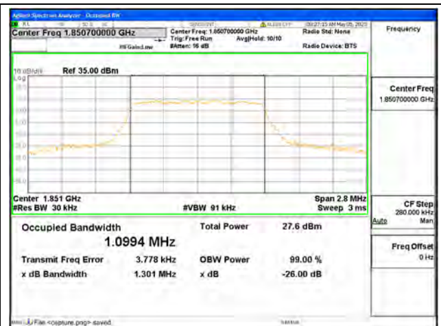
Band2 / 1.4MHz / 16QAM/ Low CH
