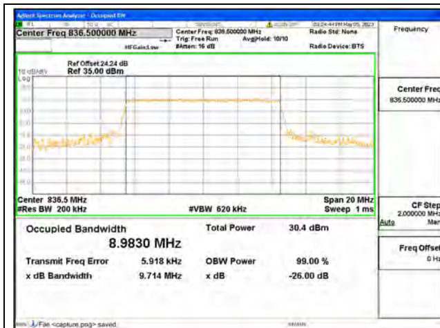
Band5 / 10MHz / QPSK/ Mid CH
