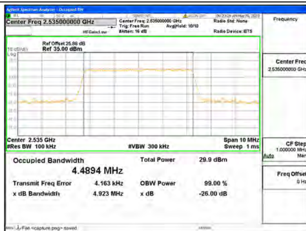
Band7 / 5MHz / 16QAM/ Mid CH
