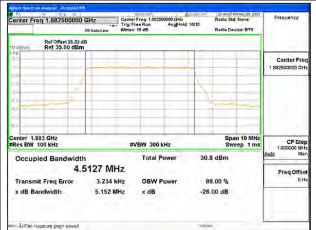
Band25 / 5MHz / QPSK/ Mid CH
