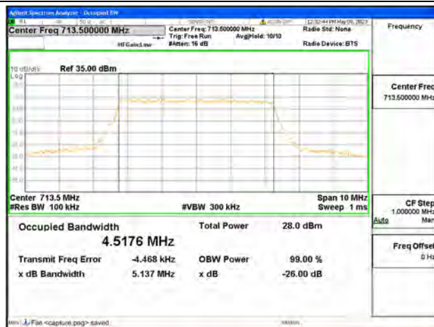
Band12 / 5MHz / 64QAM/ High CH
