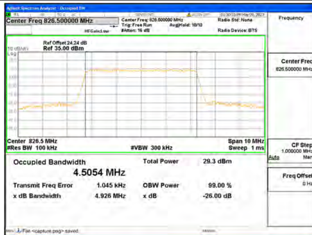
Band26 Part22 / 5MHz / 64QAM/ Low CH
