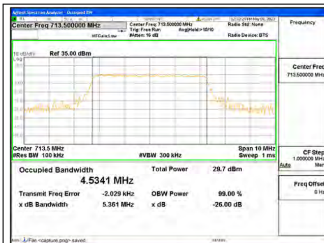
Band12 / 5MHz / QPSK/ High CH
