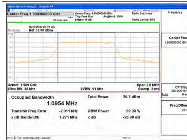
Band2 / 1.4MHz / QPSK/ High CH
