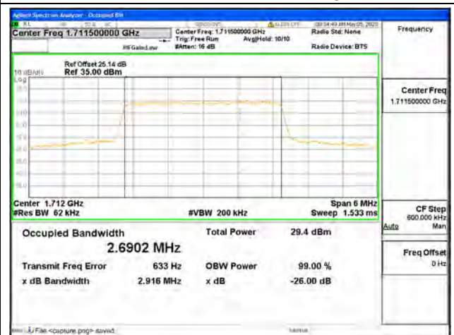
Band4 / 3MHz / QPSK/ Low CH
