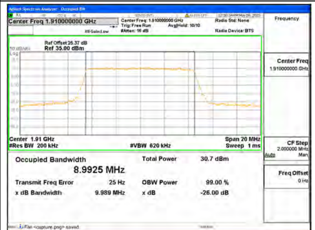
Band25 / 10MHz / QPSK/ High CH
