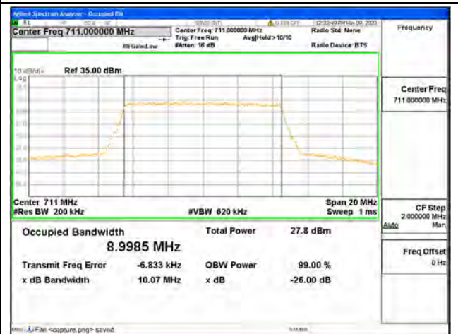
Band12 / 10MHz / 64QAM/ High CH
