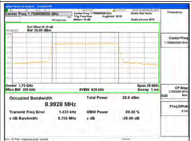
Band4 / 10MHz / QPSK/ High CH
