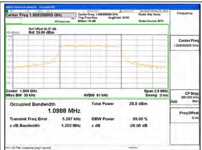
Band2 / 1.4MHz / 16QAM/ High CH
