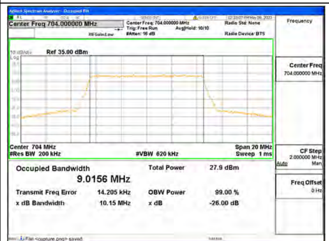
Band12 / 10MHz / 64QAM/ Low CH
