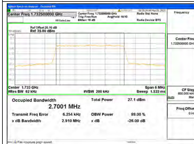
Band4 / 3MHz / 64QAM/ Mid CH
