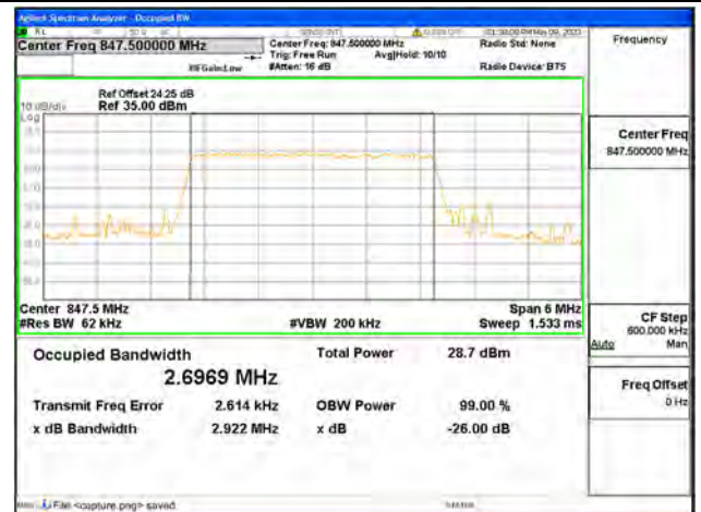
Band26 Part22 / 3MHz / 64QAM/ High CH
