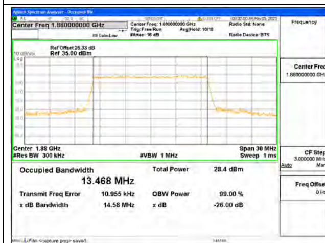
Band2 / 15MHz / 16QAM/ Mid CH
