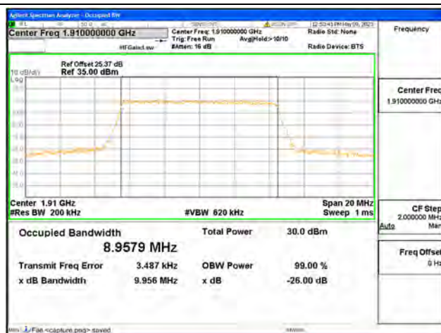
Band25 / 10MHz / 16QAM/ High CH
