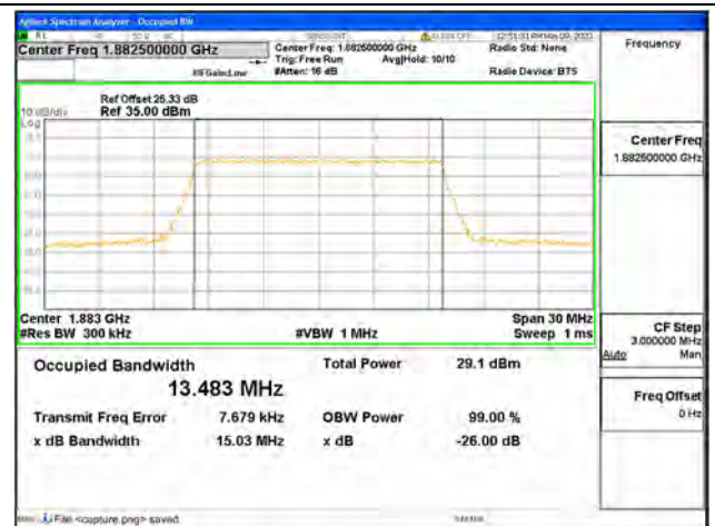
Band25 / 15MHz / 64QAM/ Mid CH
