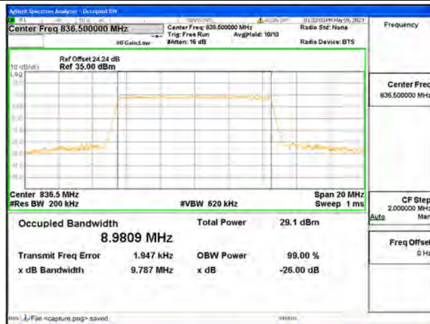
Band26 Part22 / 10MHz / 64QAM/ Mid CH
