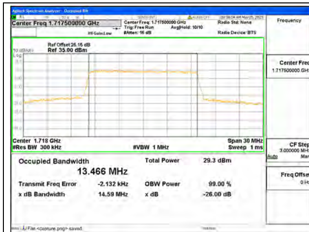
Band4 / 15MHz / QPSK/ Low CH
