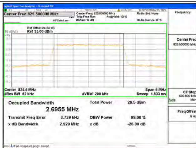
Band5 / 3MHz / 16QAM/ Low CH
