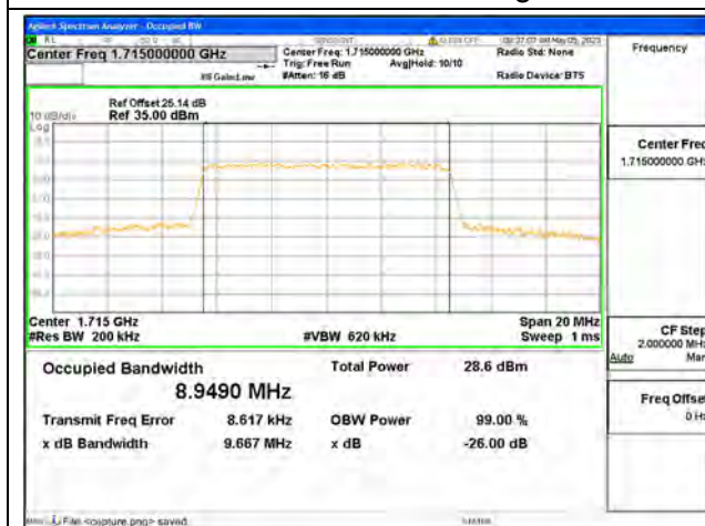
Band4 / 10MHz / 16QAM/ Low CH
