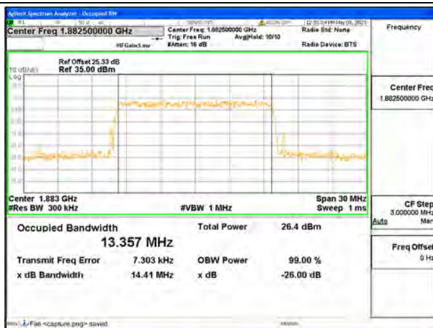
Band25 / 15MHz / 16QAM/ Mid CH
