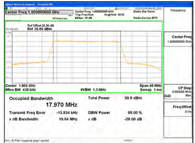
Band25 / 20MHz / QPSK/ High CH
