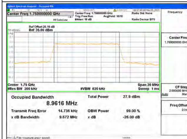
Band4 / 10MHz / 16QAM/ High CH
