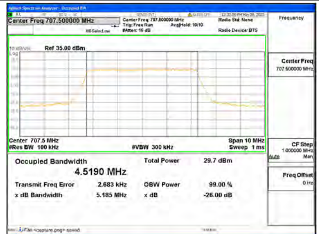
Band12 / 5MHz / QPSK/ Mid CH
