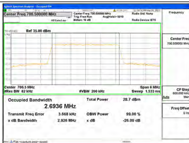
Band12 / 3MHz / 16QAM/ Low CH
