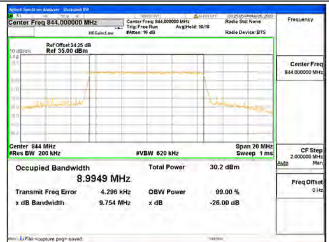
Band5 / 10MHz / QPSK/ High CH
