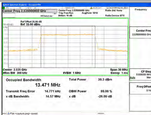
Band7 / 15MHz / 16QAM/ Mid CH
