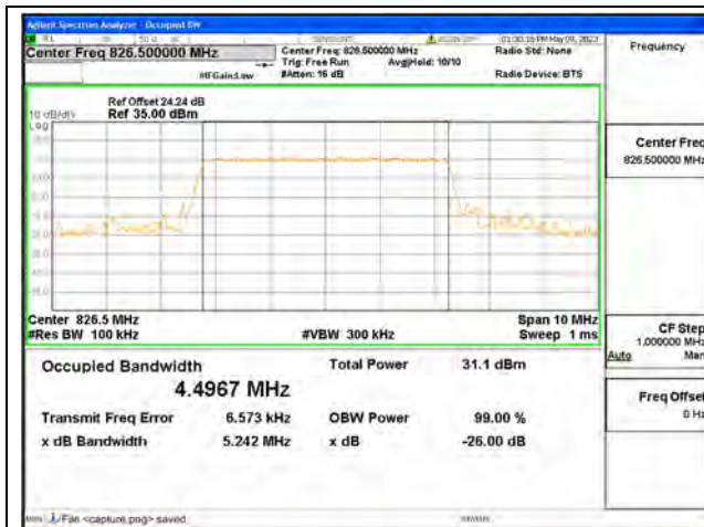
Band26 Part22 / 5MHz / QPSK/ Low CH
