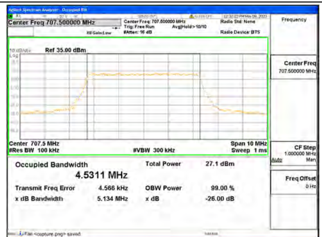
Band12 / 5MHz / 64QAM/ Mid CH
