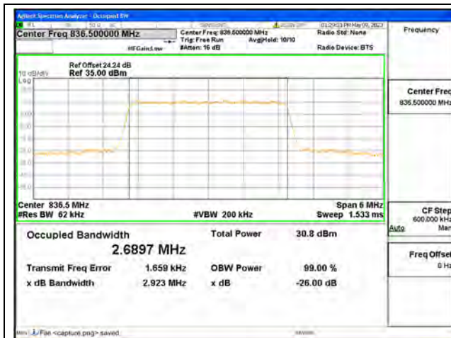
Band26 Part22 / 3MHz / QPSK/ Mid CH
