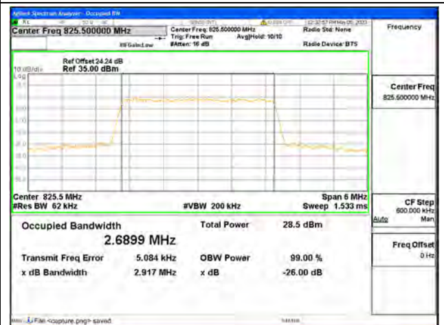
Band5 / 3MHz / 64QAM/ Low CH
