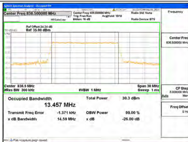
Band26 Part22 / 15MHz / 16QAM/ Mid CH
