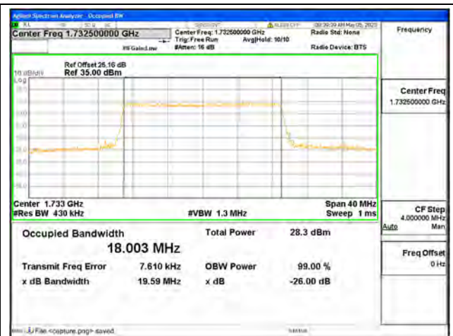
Band4 / 20MHz / 16QAM/ Mid CH
