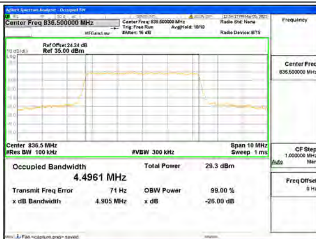
Band5 / 5MHz / 16QAM/ Mid CH
