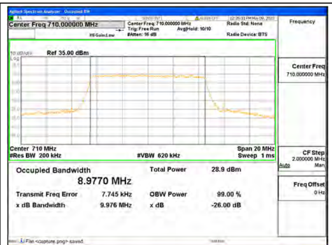
Band17 / 10MHz / 16QAM/ Mid CH
