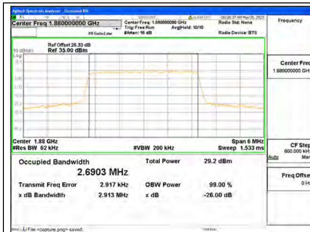
Band2 / 3MHz / QPSK/ Mid CH
