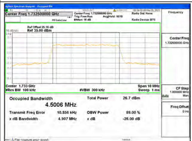
Band4 / 5MHz / 64QAM/ Mid CH
