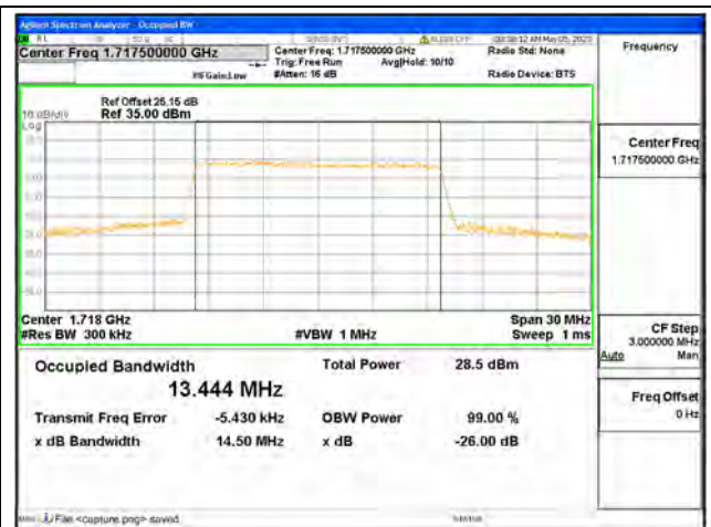
Band4 / 15MHz / 16QAM/ Low CH
