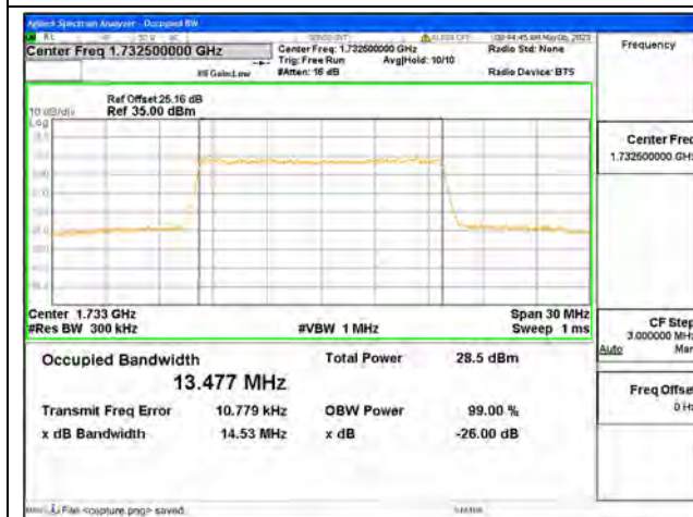
Band4 / 15MHz / 16QAM/ Mid CH
