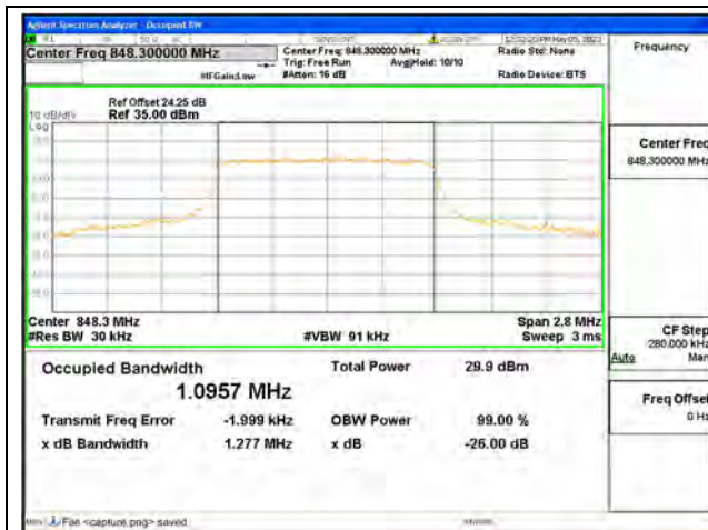
Band5 / 1.4MHz / QPSK/ High CH
