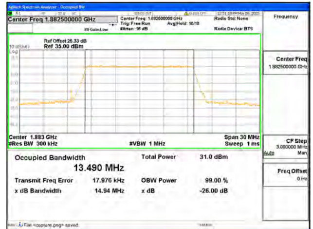
Band25 / 15MHz / QPSK/ Mid CH
