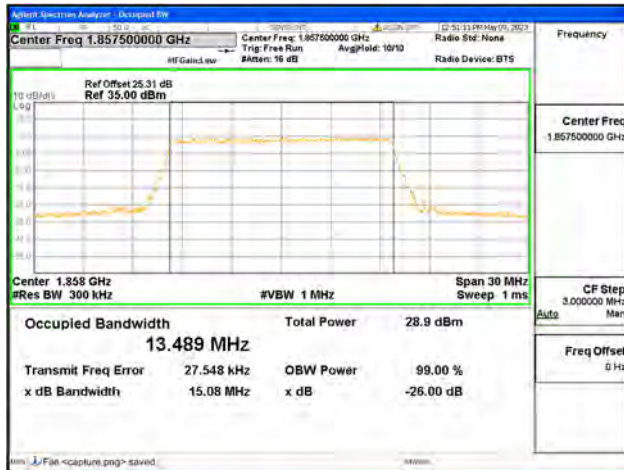
Band25 / 15MHz / 64QAM/ Low CH
