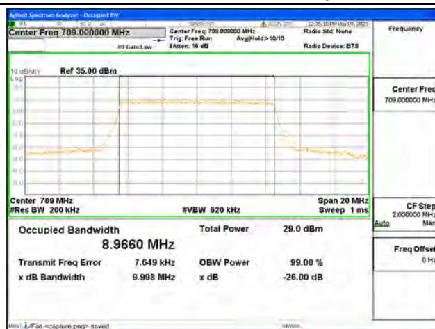
Band17 / 10MHz / 16QAM/ Low CH
