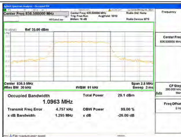
Band5 / 1.4MHz / 16QAM/ Mid CH
