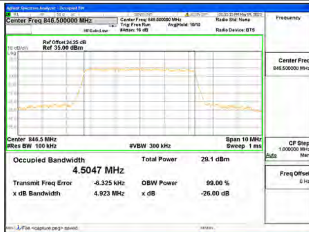
Band26 Part22 / 5MHz / 64QAM/ High CH
