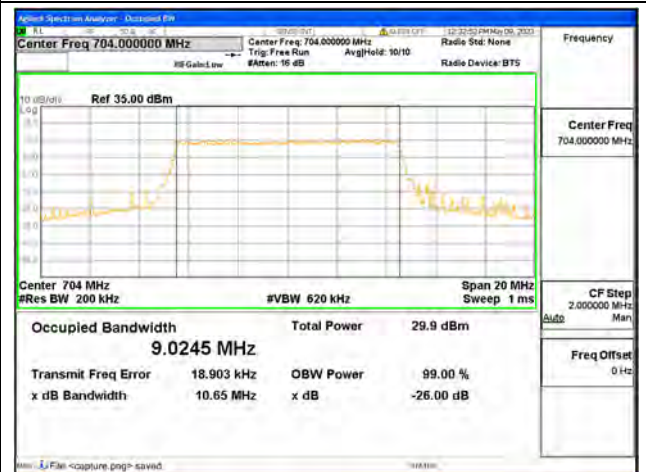
Band12 / 10MHz / QPSK/ Low CH
