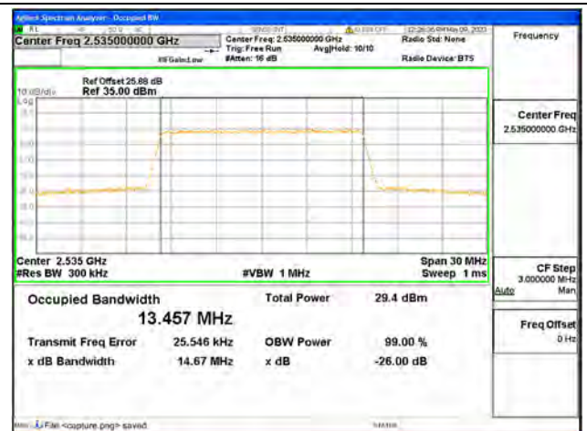
Band7 / 15MHz / 64QAM/ Mid CH
