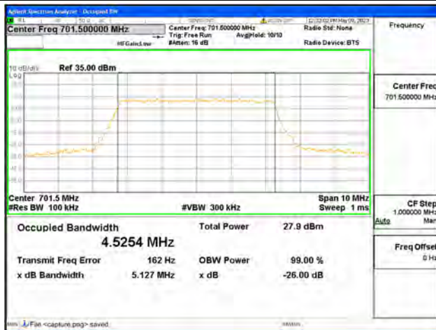
Band12 / 5MHz / 64QAM/ Low CH
