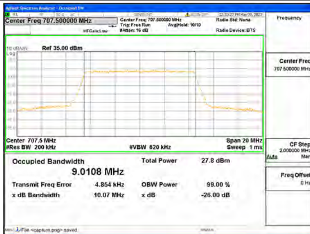
Band12 / 10MHz / 64QAM/ Mid CH
