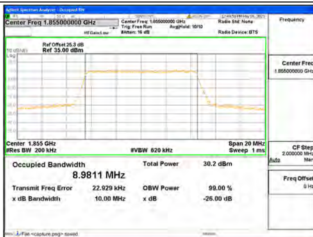
Band25 / 10MHz / 16QAM/ Low CH
