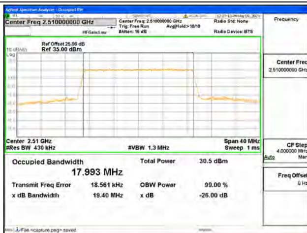
Band7 / 20MHz / 16QAM/ Low CH
