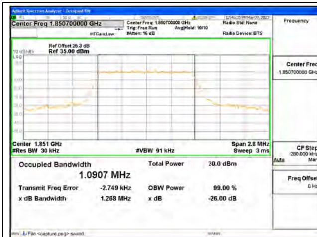
Band25 / 1.4MHz / QPSK/ Low CH
