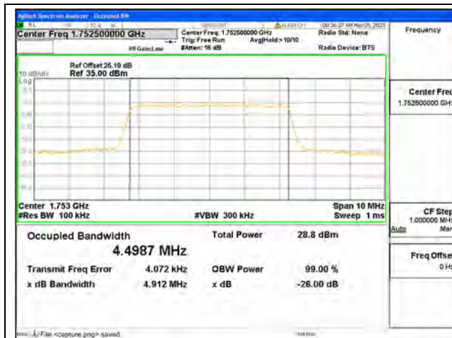
Band4 / 5MHz / QPSK/ High CH
