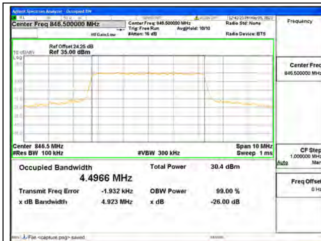
Band5 / 5MHz / QPSK/ High CH
