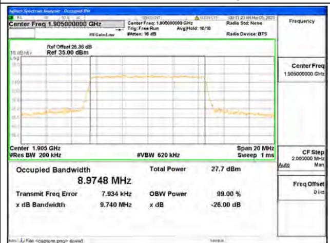
Band2 / 10MHz / 64QAM/ High CH
