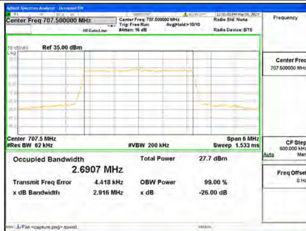
Band12 / 3MHz / 64QAM/ Mid CH
