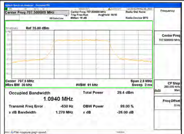
Band12 / 1.4MHz / QPSK/ Mid CH
