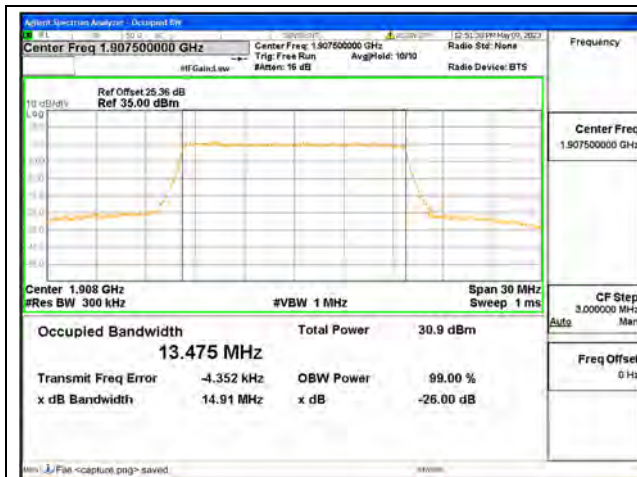
Band25 / 15MHz / QPSK/ High CH
