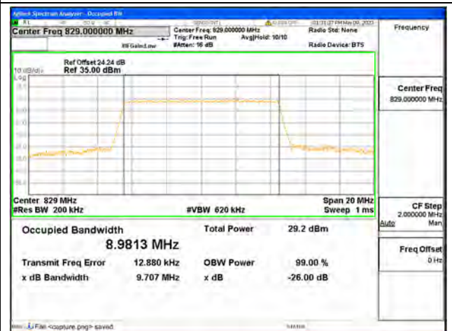
Band26 Part22 / 10MHz / 64QAM/ Low CH
