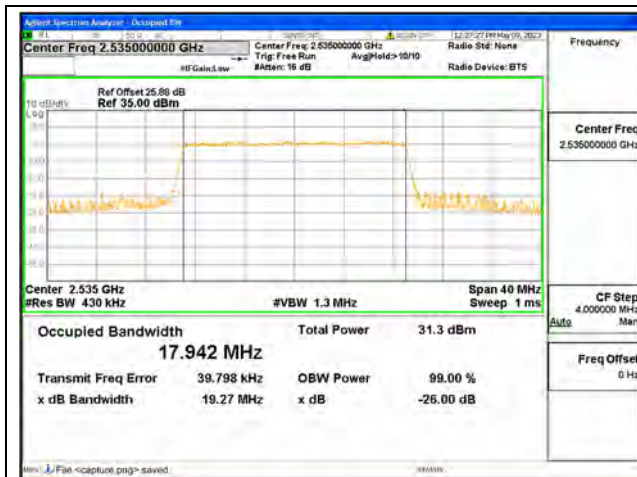
Band7 / 20MHz / QPSK/ Mid CH
