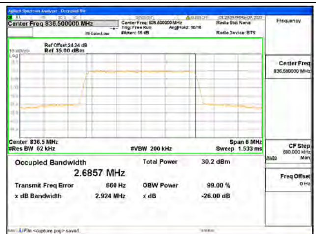
Band26 Part22 / 3MHz / 16QAM/ Mid CH
