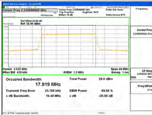
Band7 / 20MHz / 64QAM/ Mid CH
