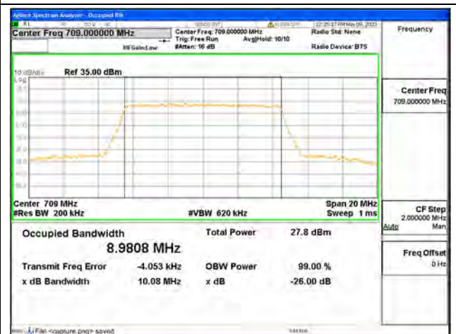
Band17 / 10MHz / 64QAM/ Low CH
