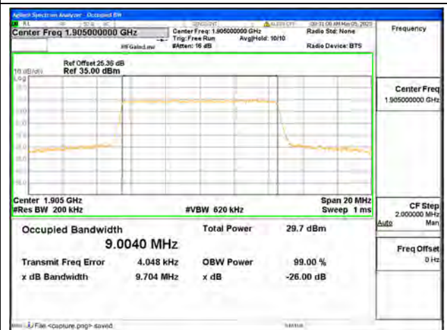
Band2 / 10MHz / QPSK/ High CH
