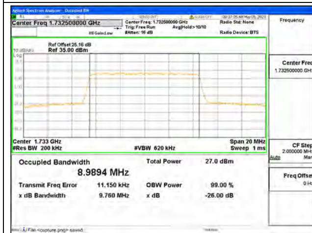
Band4 / 10MHz / 64QAM/ Mid CH
