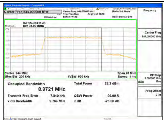
Band5 / 10MHz / 64QAM/ High CH
