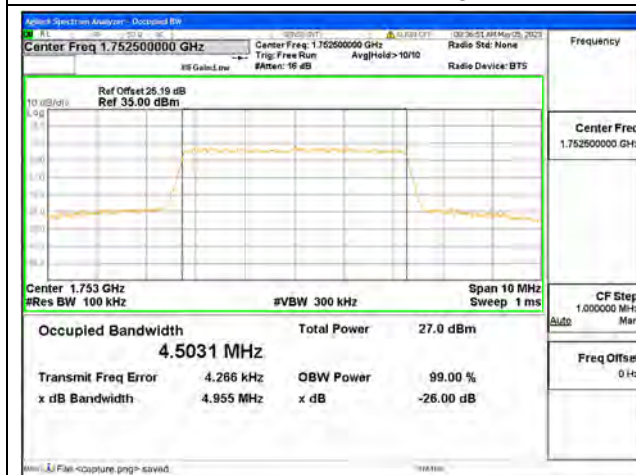
Band4 / 5MHz / 64QAM/ High CH
