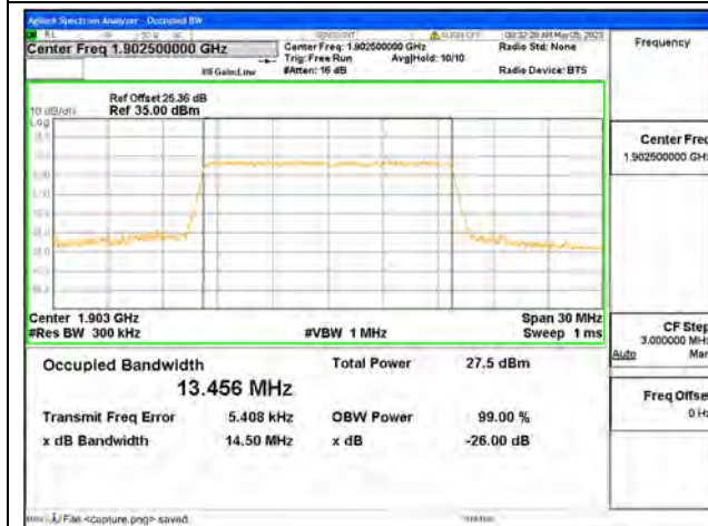
Band2 / 15MHz / 64QAM / High CH
