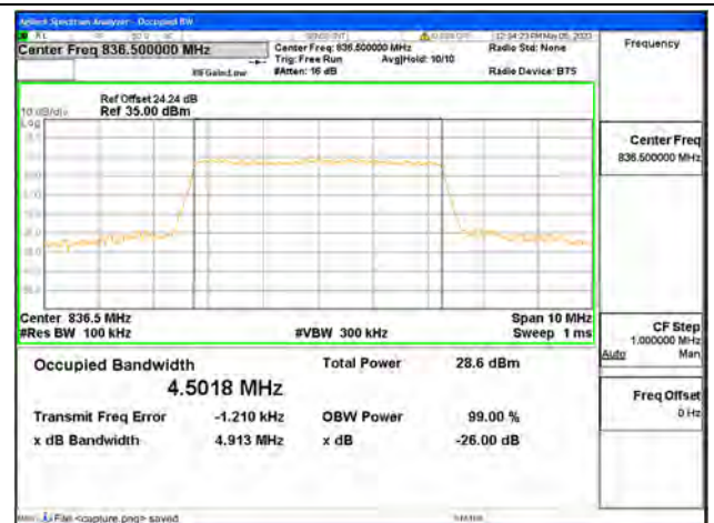
Band5 / 5MHz / 64QAM/ Mid CH
