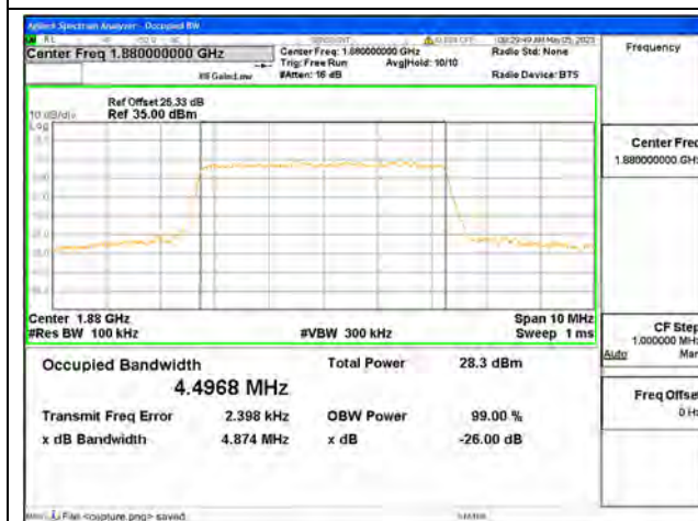
Band2 / 5MHz / 16QAM/ Mid CH
