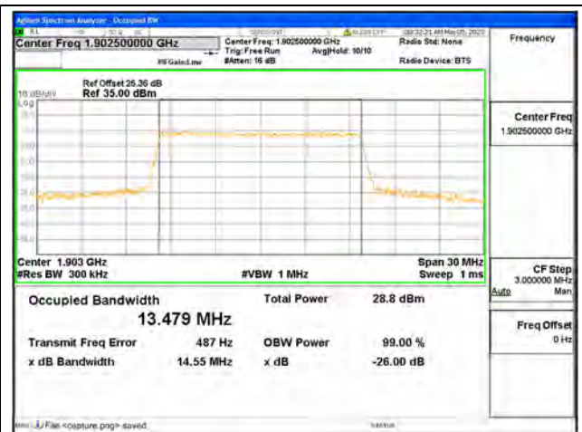
Band2 / 15MHz / 16QAM / High CH
