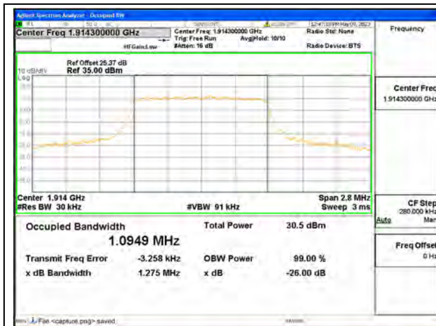
Band25 / 1.4MHz / QPSK/ High CH
