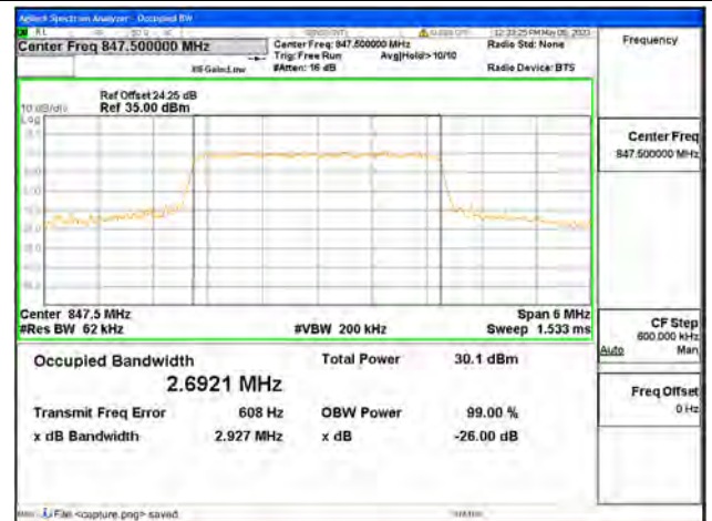
Band5 / 3MHz / QPSK/ High CH
