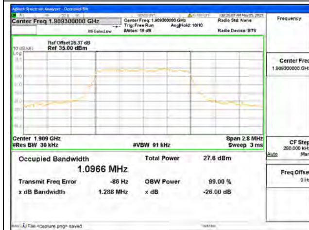
Band2 / 1.4MHz / 64QAM/ High CH
