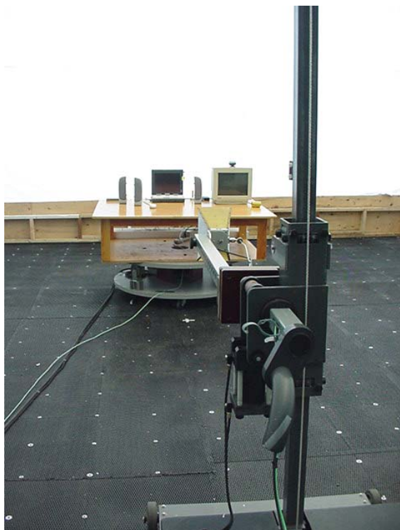
Photograph E.7-3 - Front of Radiated Emission Setup with attached swivel dipole antenna
