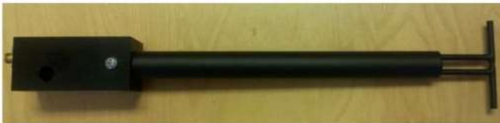
**Figure 1 – MVG COMOSAR Validation Dipole**
