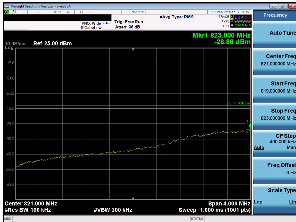
Plot 7-119. Lower Extended Band Edge Plot (Band 5 - 3.0MHz QPSK - Full RB Configuration)
