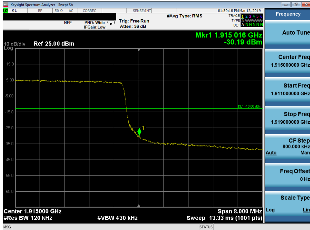
Plot 7-176. Upper Band Edge Plot (Band 25 - 10.0MHz QPSK - Full RB Configuration)
