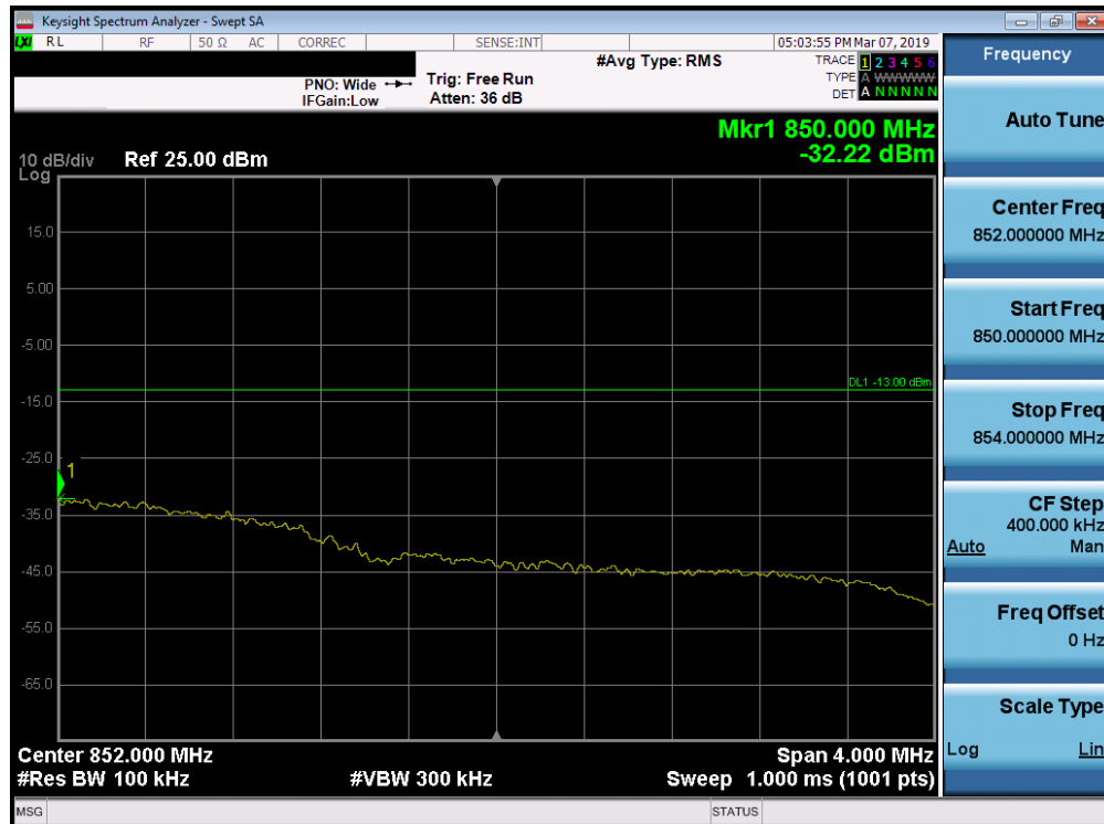
Plot 7-121. Upper Extended Band Edge Plot (Band 5 - 3.0MHz QPSK - Full RB Configuration)
