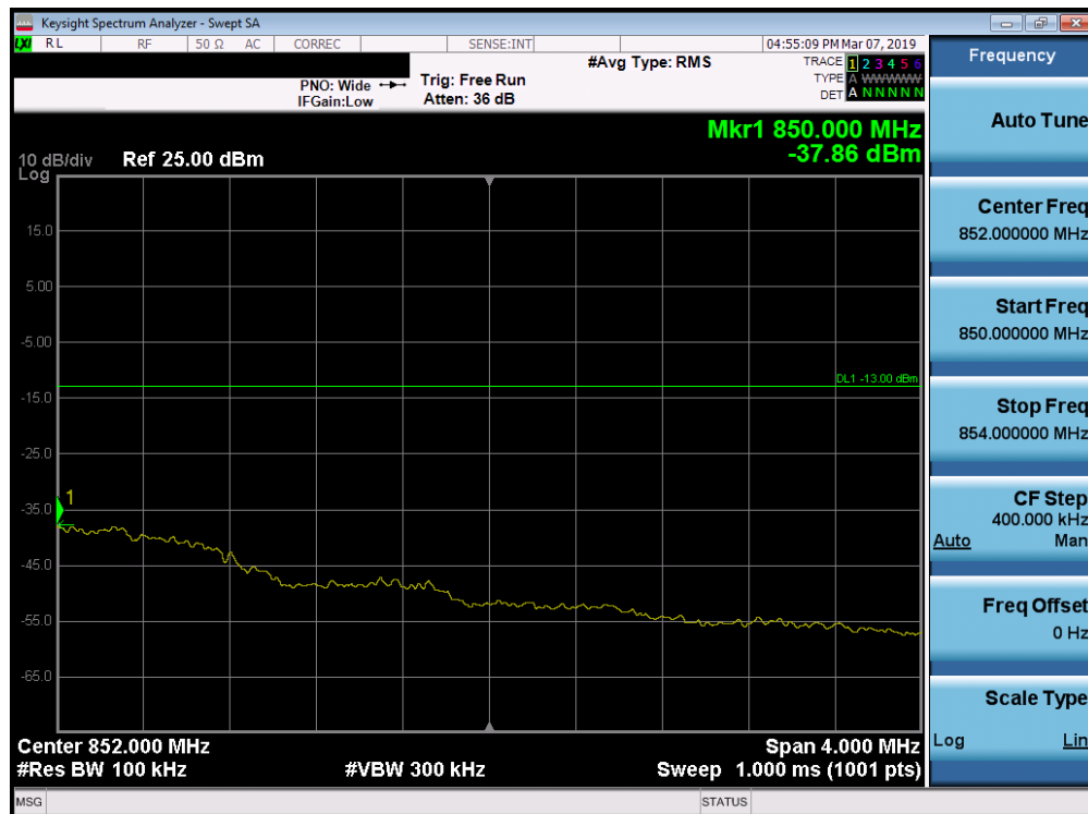
Plot 7-117. Upper Extended Band Edge Plot (Band 5 - 1.4MHz QPSK - Full RB Configuration)
