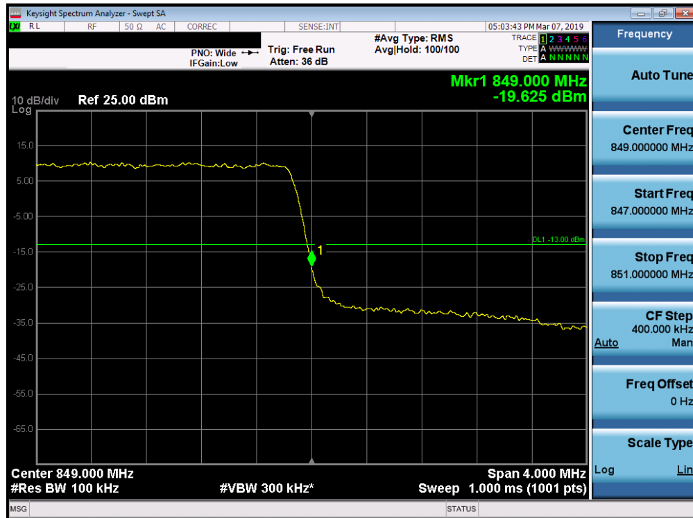
Plot 7-120. Upper Band Edge Plot (Band 5 - 3.0MHz QPSK - Full RB Configuration)
