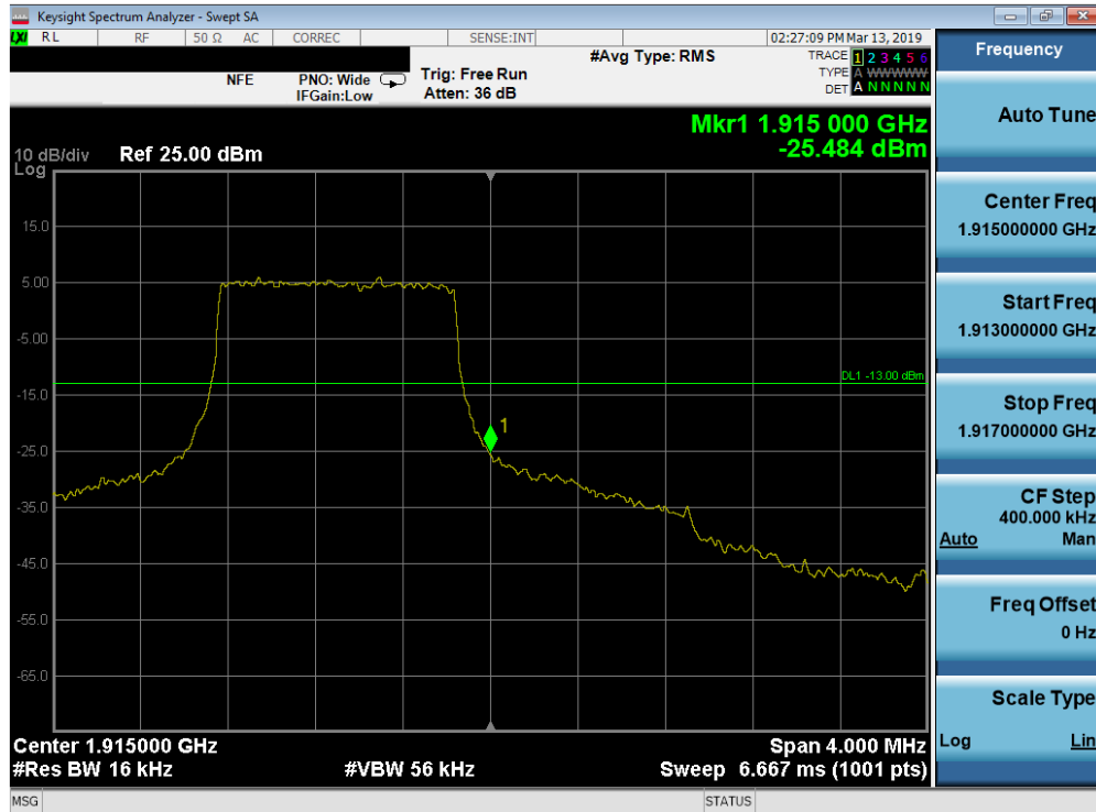
Plot 7-158. Upper Band Edge Plot (Band 25 - 1.4MHz QPSK - Full RB Configuration)
