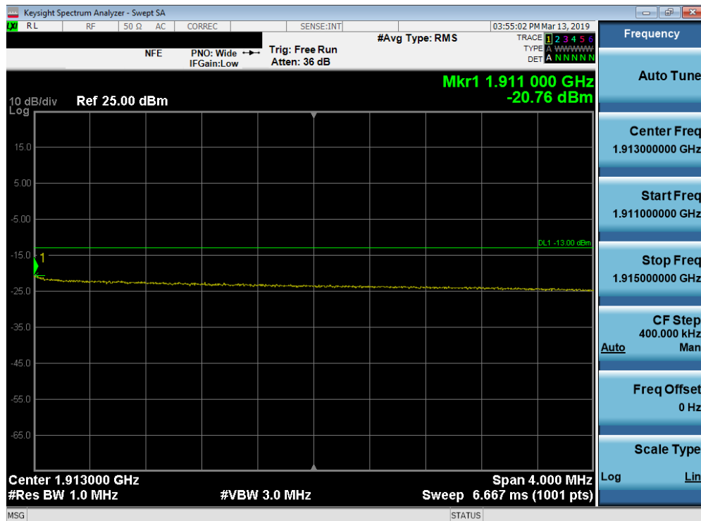
Plot 7-175. Upper Extended Band Edge Plot (Band 2 - 10.0MHz QPSK - Full RB Configuration)
