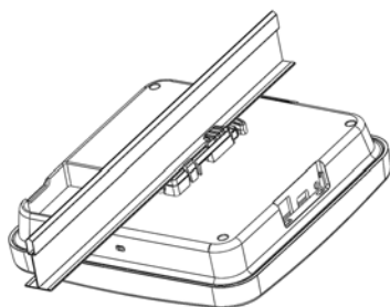
5. Ensure all screws on device are snapped in to the grooves on the bracket
