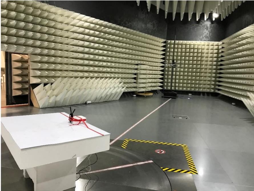
**Photograph 1: Test Set Up Radiated Emissions 30 – 1000 MHz**
