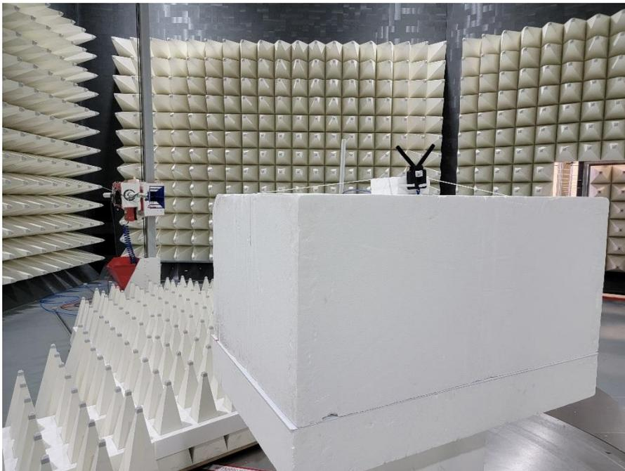
**Photograph 2: Test Set Up Radiated Emissions 1 – 17 GHz**
