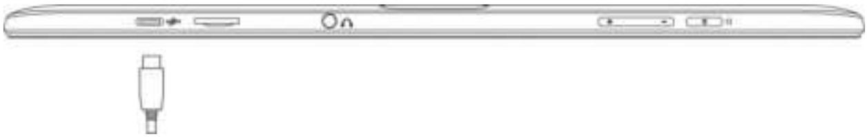
This device supports external USB devices for extending the memory size, or a USB-C Thumb Drive. Insert a USB cable (not included) from the external device into the USB-C port on the side of unit. Insert the other side to the device.
