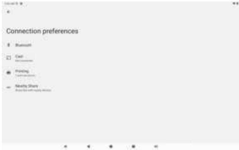
**C: Tap “Bluetooth”, and turn on the “Bluetooth” to “ON” position by sliding the “ON/OFF” button to the right,**
