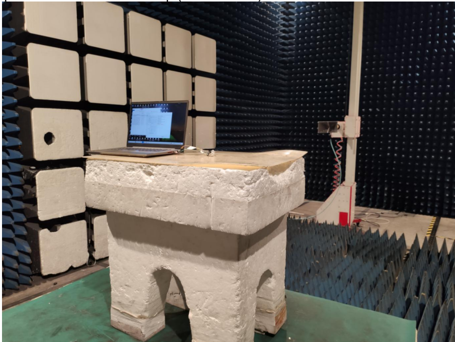
Spurious Emission Test Setup (Above 1GHz)
