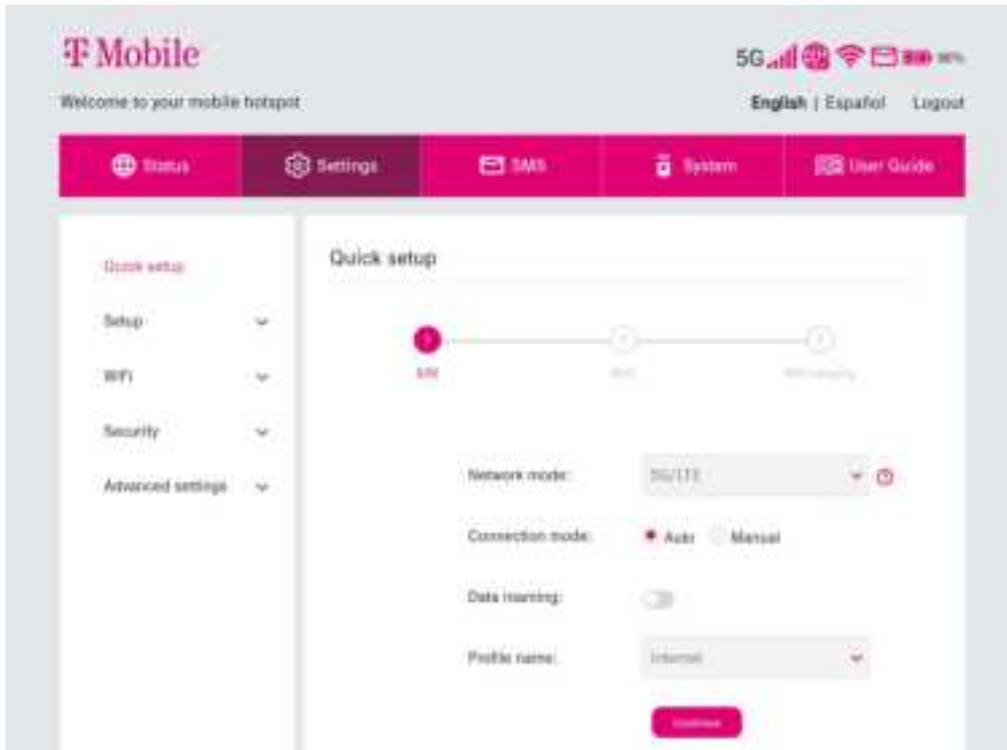
On the next page, you can change the 2.4 and 5GHz Wireless network name (SSID), SSID broadcast function or disable the Wi-Fi.
