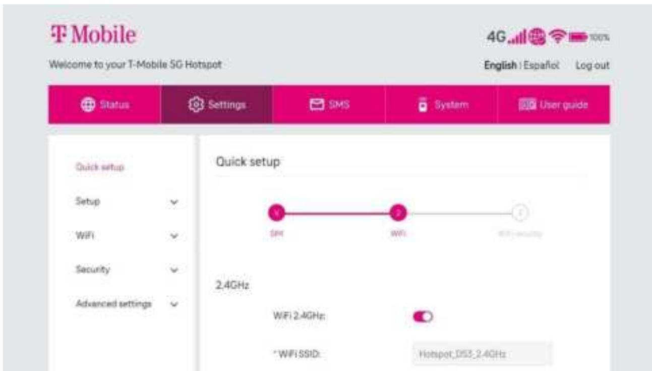
On the final page, you can setup basic Wi-Fi setting such as security settings, and Wi-Fi password.
