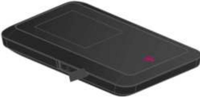
2. Insert the SIM card into the slot with the gold contacts facing downwards.
