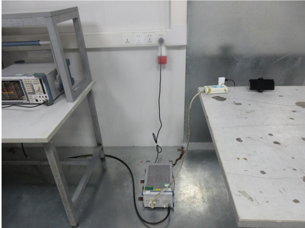
Photo of Conducted Emission Measurement
