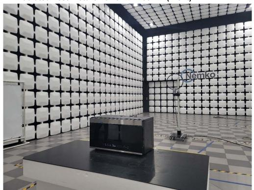
■ Radiated Test Picture : 0.15 M₂ ~ 30 M₂ (Front)
