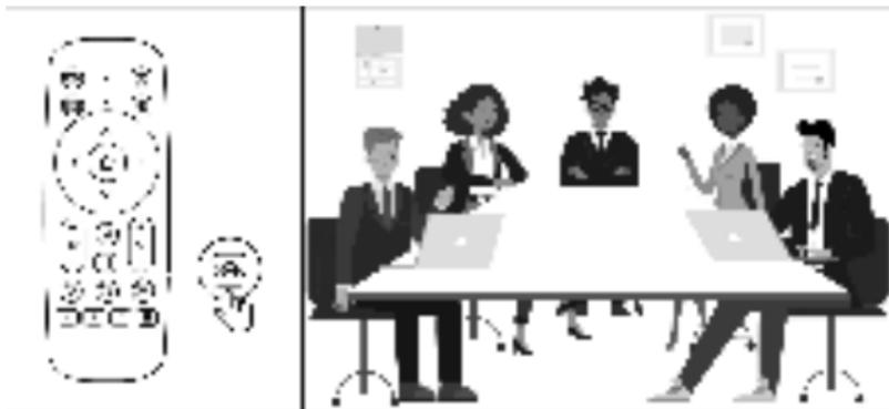
**Step 2** When the participant's position moves, the camera will automatically adjust the image using facial recognition to achieve the best composition.
