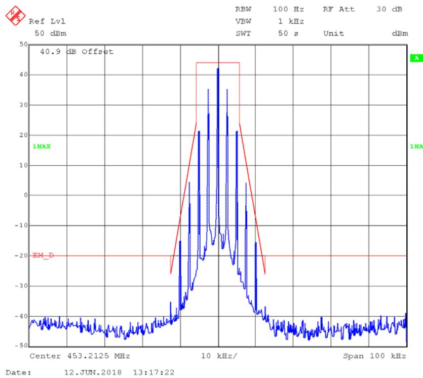
**FM,12.5kHz,Low Power - Frequency 453.2125 MHz: 99% Occupied & 26 dB Bandwidth**
