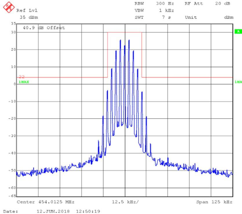
**4FSK,12.5kHz,High Power - Frequency 454.0125 MHz: 99% Occupied & 26 dB Bandwidth**
