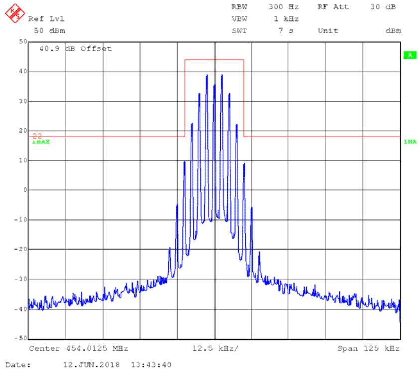
**FM,25kHz,Low Power - Frequency 454.0125 MHz: 99% Occupied & 26 dB Bandwidth**
