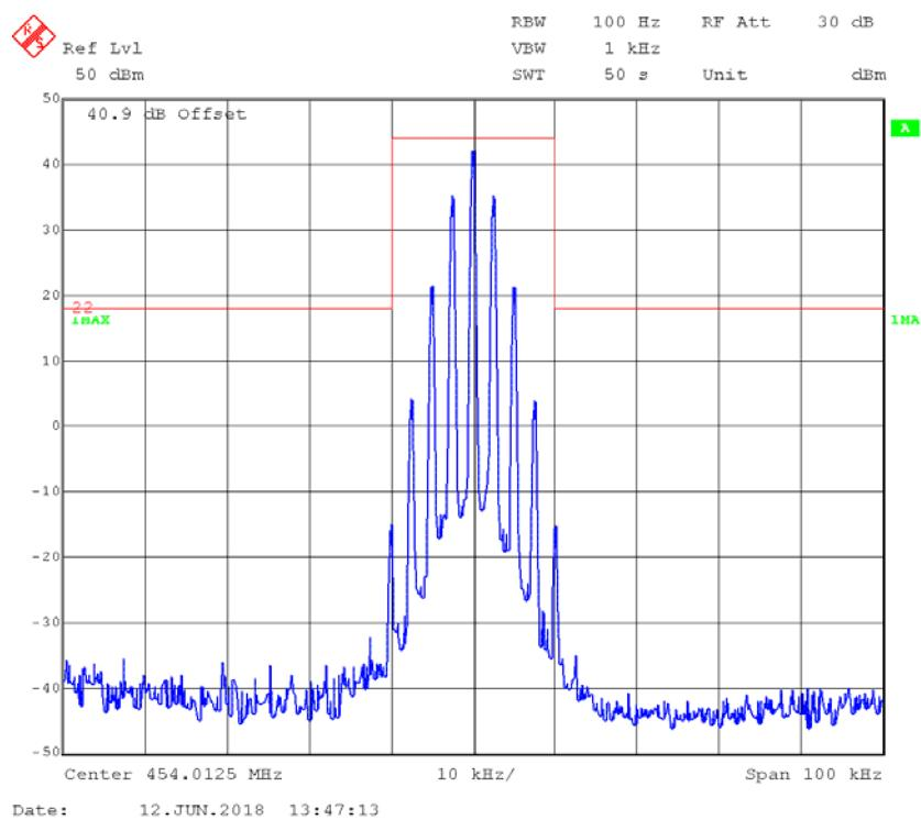
**FM,12.5kHz,Low Power - Frequency 454.0125 MHz: 99% Occupied & 26 dB Bandwidth**
