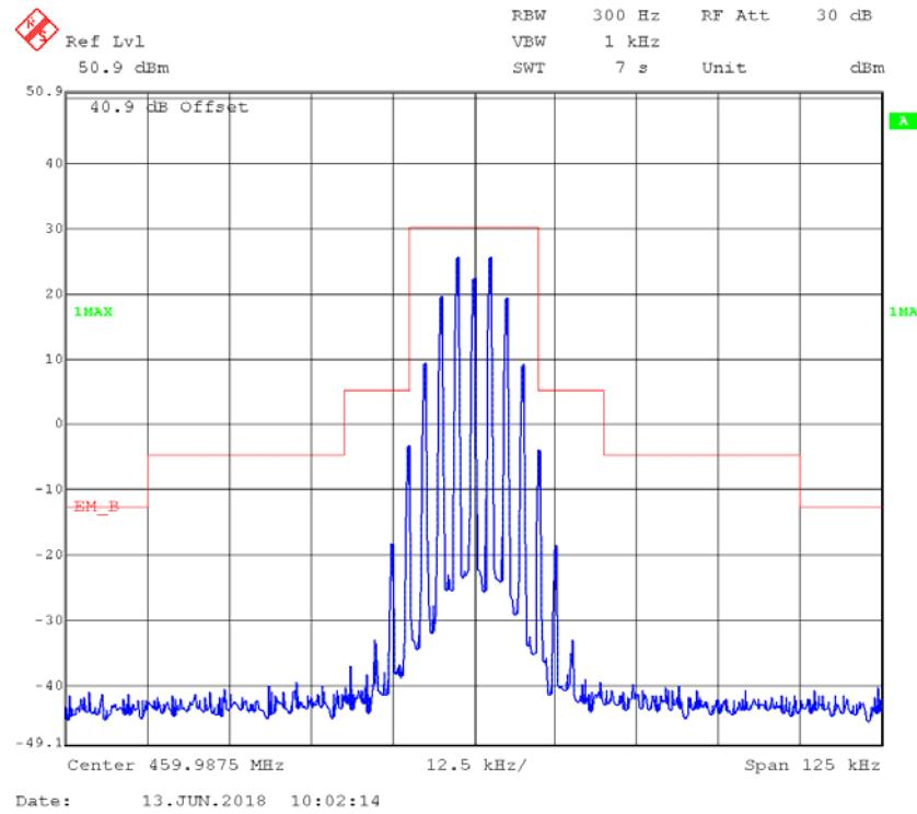
**Part 74****FM,12.5kHz,High Power - Frequency 450.03125 MHz: 99% Occupied & 26 dB Bandwidth**
