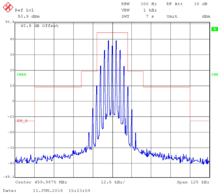
**FM,25kHz,Low Power - Frequency 459.9875 MHz MHz: 99% Occupied & 26 dB Bandwidth**
