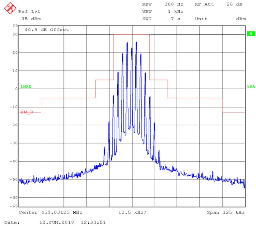
**4FSK,12.5kHz,High Power - Frequency 450.03125 MHz: 99% Occupied & 26 dB Bandwidth**
