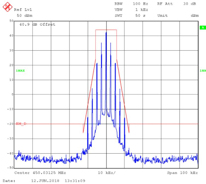
**FM,12.5kHz,Low Power - Frequency 450.03125 MHz: 99% Occupied & 26 dB Bandwidth**
