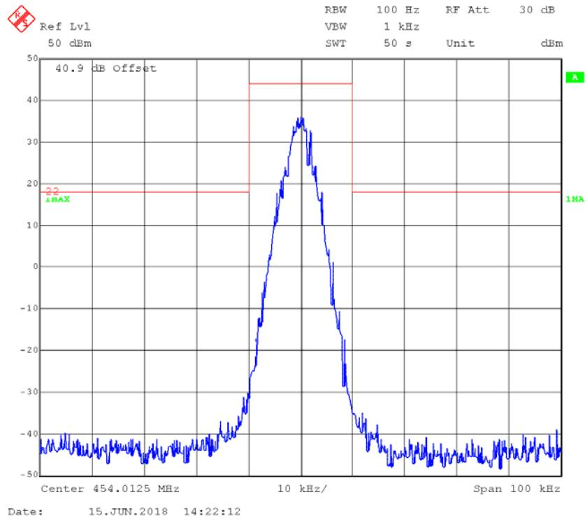
**4FSK,12.5kHz,Low Power - Frequency 454.0125 MHz: 99% Occupied & 26 dB Bandwidth**
