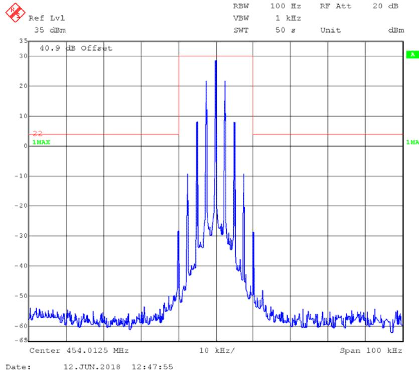
**FM,25kHz,High Power - Frequency 454.0125 MHz: 99% Occupied & 26 dB Bandwidth**
