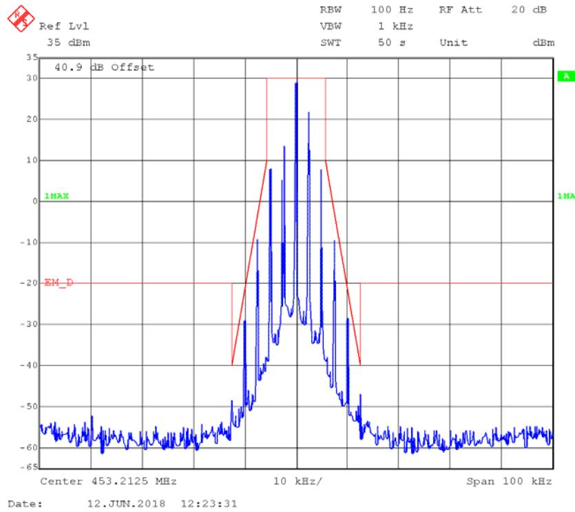
**4FSK,12.5kHz,High Power - Frequency 453.2125 MHz: 99% Occupied & 26 dB Bandwidth**
