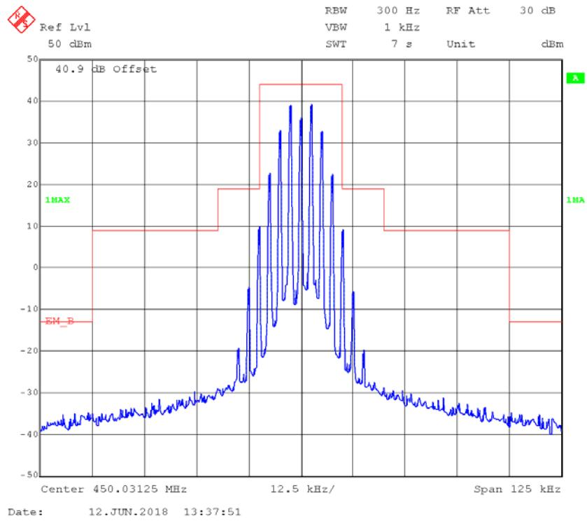
**FM,25kHz,Low Power - Frequency 450.03125 MHz: 99% Occupied & 26 dB Bandwidth**
