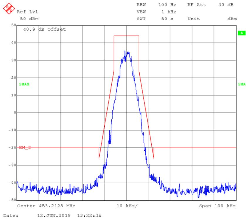
**4FSK,12.5kHz,Low Power - Frequency 453.2125 MHz: 99% Occupied & 26 dB Bandwidth**
