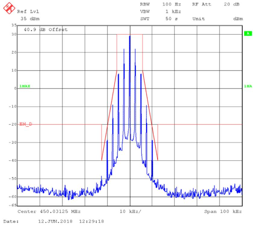
**FM,25kHz,High Power - Frequency 450.03125 MHz: 99% Occupied & 26 dB Bandwidth**
