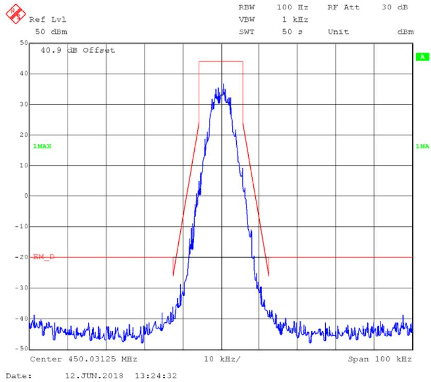
**4FSK,12.5kHz,Low Power - Frequency 450.03125 MHz: 99% Occupied & 26 dB Bandwidth**
