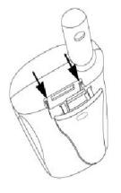
Hook the belt clip into the notch at top of the radio and slide down until it clicks into place.
