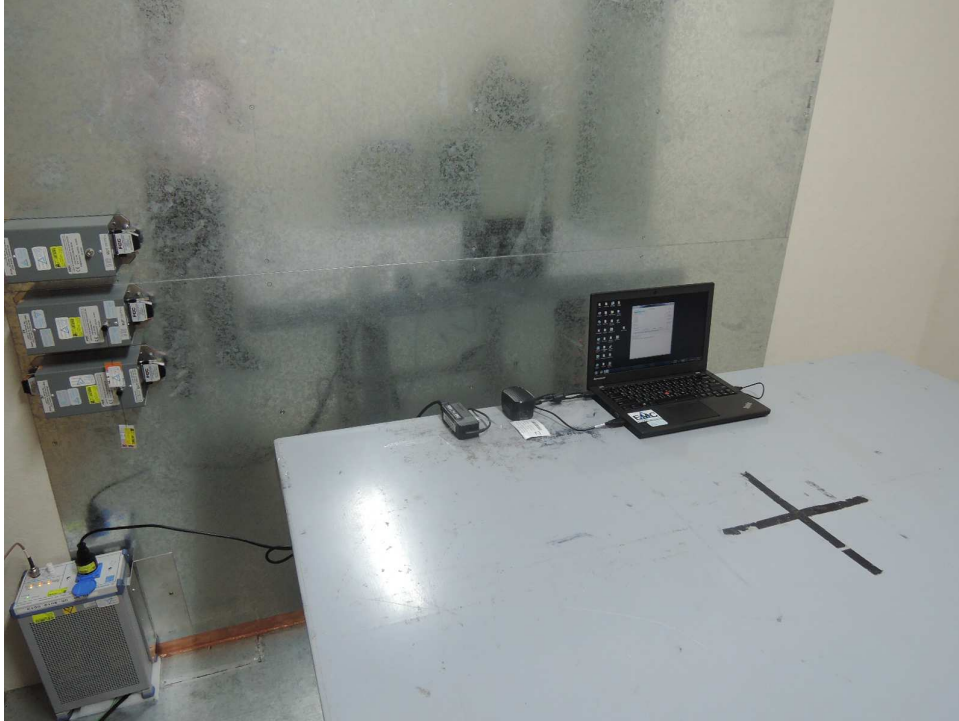
Photograph 6: Set-up for for Mains Conducted testing Front
