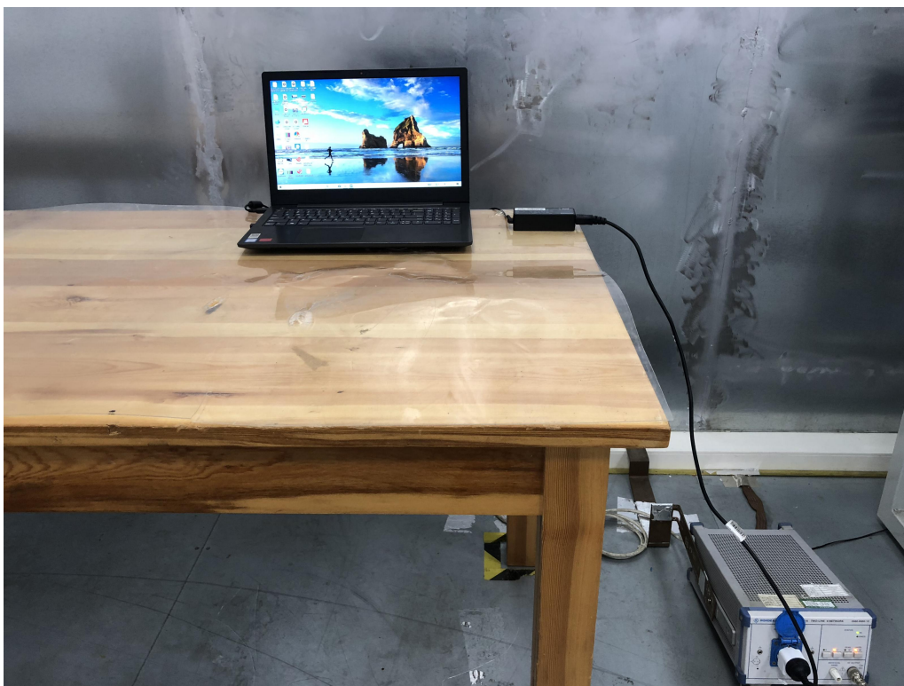
Test Setup Photo of Conducted Emission Measurement
