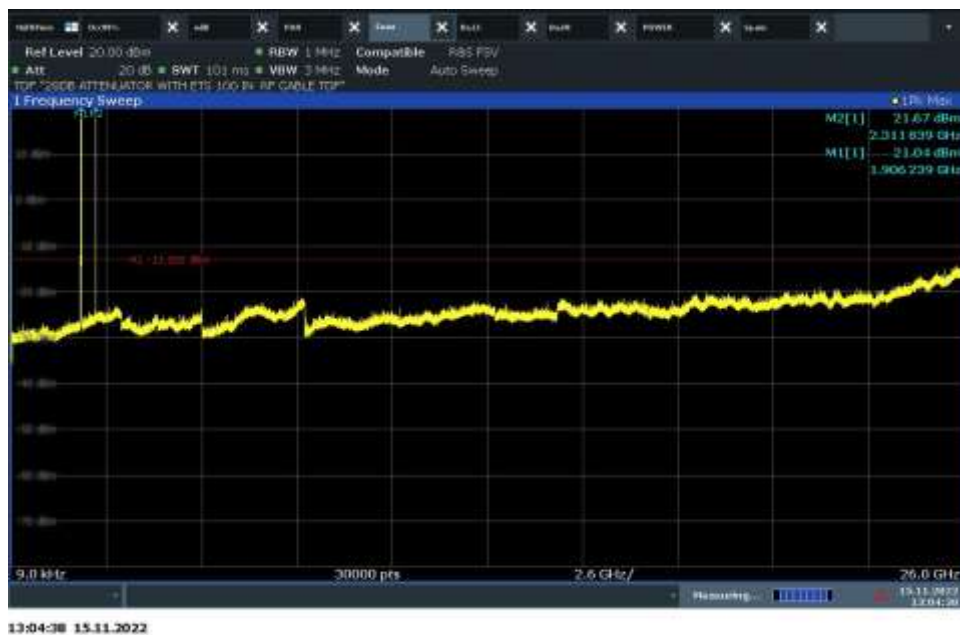
2 Bands per antenna Port 2 conducted Spurious Emissions Antenna Port 1 Uplink: WCDMA Band 5 5MHz BW Mid Ch & LTE Band 12 10MHz BW Low Ch
