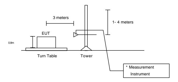
\* 30-1000 MHz, Rohde & Schwarz ESI40 receiver or 1-10 GHz, ESI40 with preamplifier and high-pass filter
