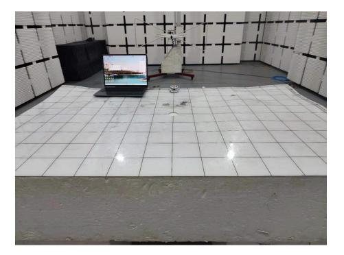
Set-up for Radiated Spurious Emission, Below 1GHz
