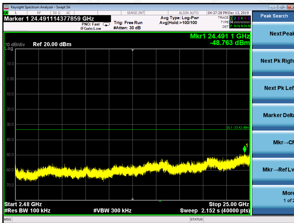
TEST PLOT OF OUT OF BAND EMISSIONS THE WORST CASE OF (802.11n20 with data rate 6.5) FOR MODULATION IN MIDDLE CHANNEL
