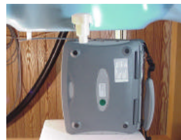
Body SAR Test Setup with 2.0cm separation distance
