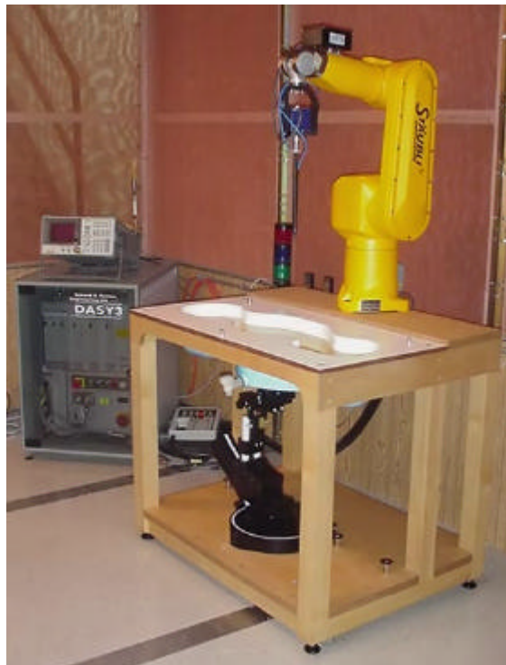
DASY3 SAR Measurement System
