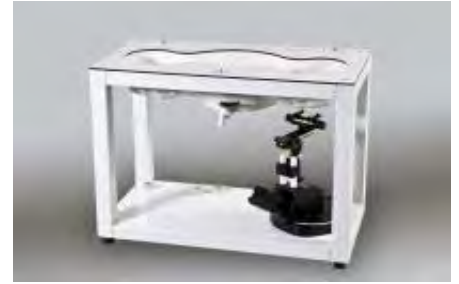
Figure E.5.1 SAM Twin Phantom
