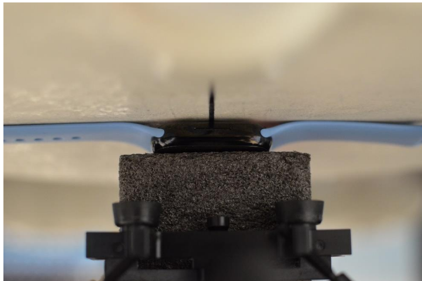
SAR Test Setup Photo 13: Stainless Steel with Sport Wristband, Extremity, Back Side at 0.0 cm
