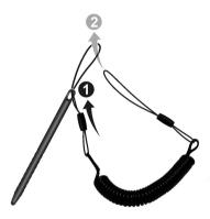
2. Insert the other loop end to the tether hole on the Tablet PC (as indicated by **1** below). Then, insert the stylus end through the loop (as indicated by **2** below) and pull it tight.
