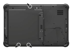
The bottom I/O cover must be secured to F110-Ex with two screws. While not in an Ex-hazardous area, you can remove this cover in order to access any connector behind it.
