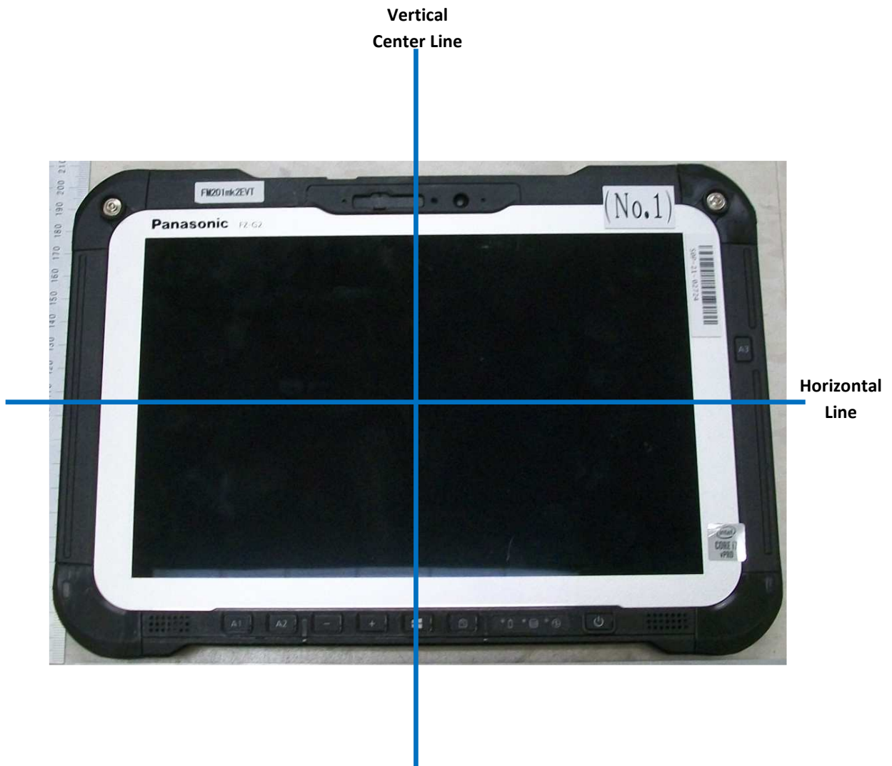
Photograph 6: Handset Vertical and Horizontal Reference Lines
