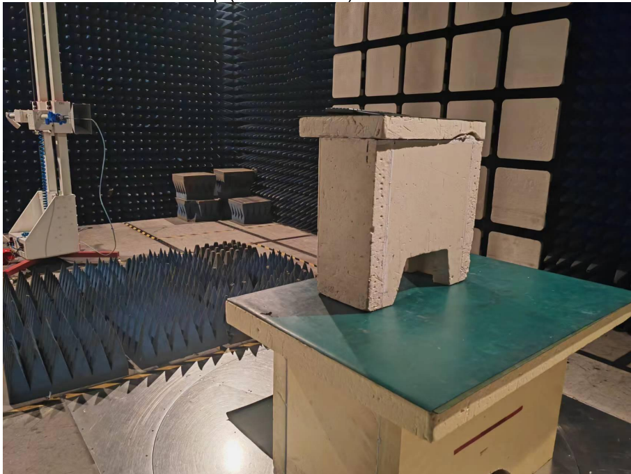
Spurious Emission Test Setup (30MHz-1GHz)
