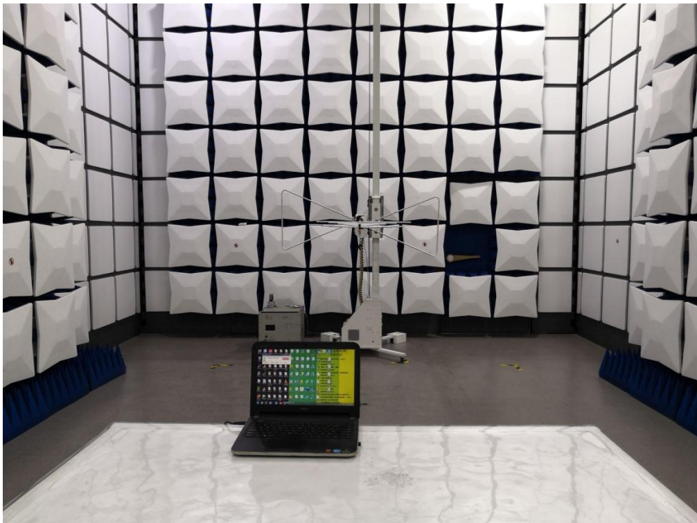
FCC RADIATED EMISSION TEST SETUP BELOW 1GHZ
