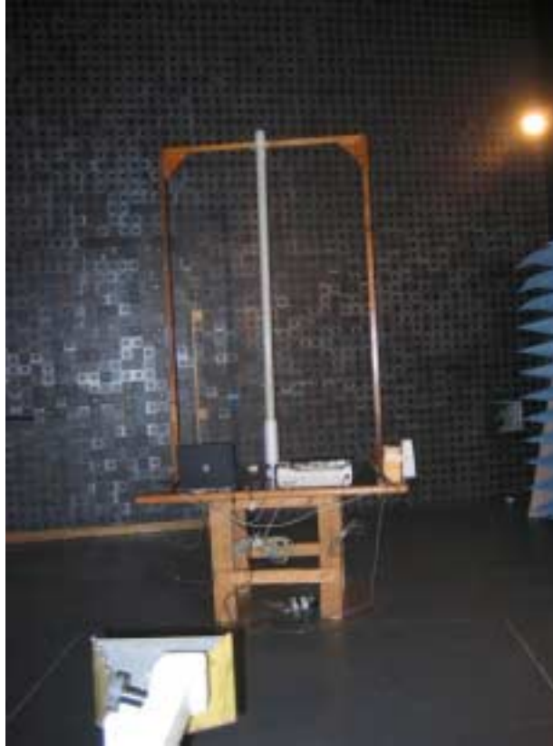
Photograph No.9 Spurious emissions measurement setup in the anechoic chamber above 1 GHz, EUT with omni-directional
