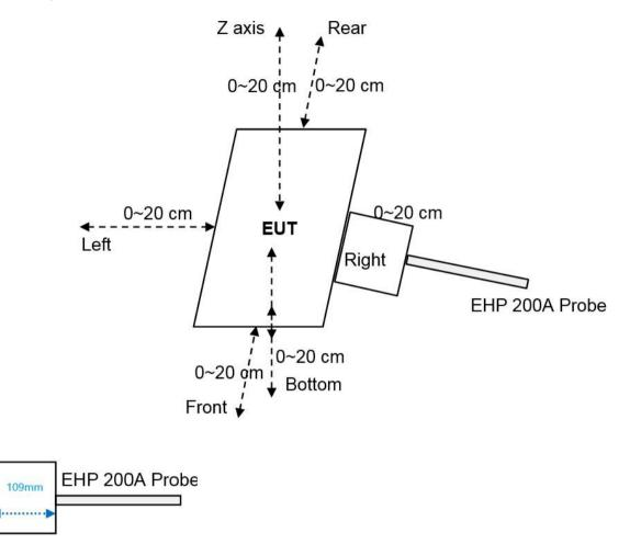
Notes: The EHP 200A Probe has a diameter of 10.9cm and a radius of 5.45cm.
