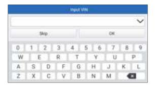
Input the VIN and tap "OK"; the system will automatically identify the vehicle model.
