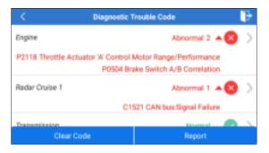
The system with fault codes will be displayed in red ( $\bigotimes$ ). The system with no fault codes will be displayed in green ( $\checkmark$ ).
