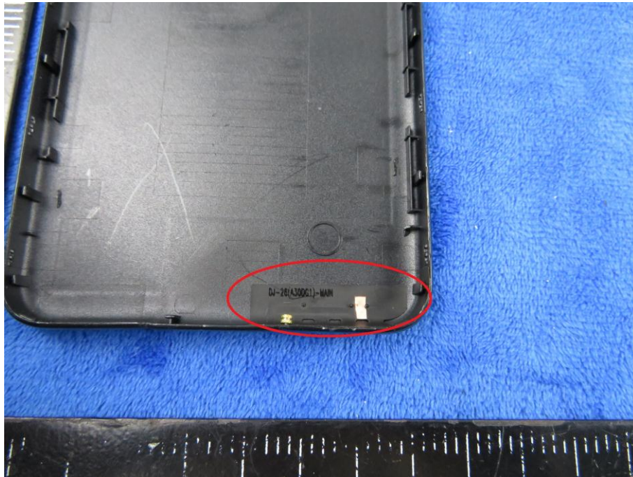
GSM/PCS/UMTS-FDD - Antenna View
