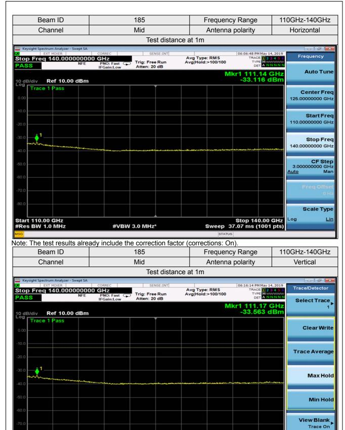
Note: The test results already include the correction factor (corrections: On).
