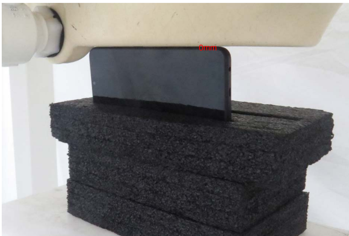
Picture 16: Right Edge, the distance from handset to the bottom of the Phantom is 0mm
