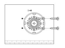
Secure the mounting bracket to the wall by driving the self-tapping screws into the anchors. Make sure that the shoulders of the mounting bracket are
