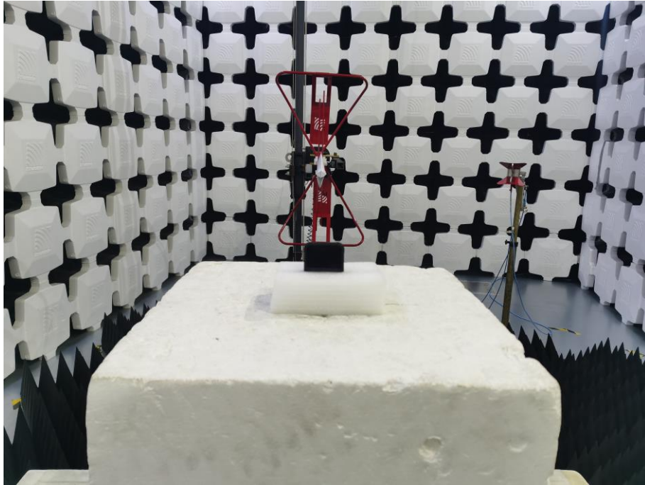
11. Radiated Emissions (Part 15C&15E, 1GHz -18GHz)
