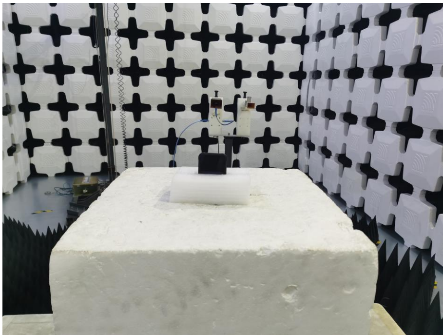
12. Radiated Emissions (Part 15C&15E, 26.5GHz-40GHz)
