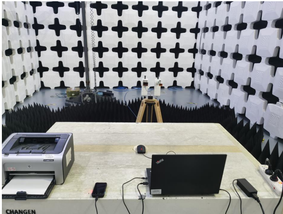
3. Radiated Emissions (Part 15B Data Transfer ,18GHz-26.5GHz)
