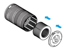
5. Turn the base cover clockwise from **OPEN** position to **LOCK** position, you will hear a "click" sound, the base cover is fastened.
