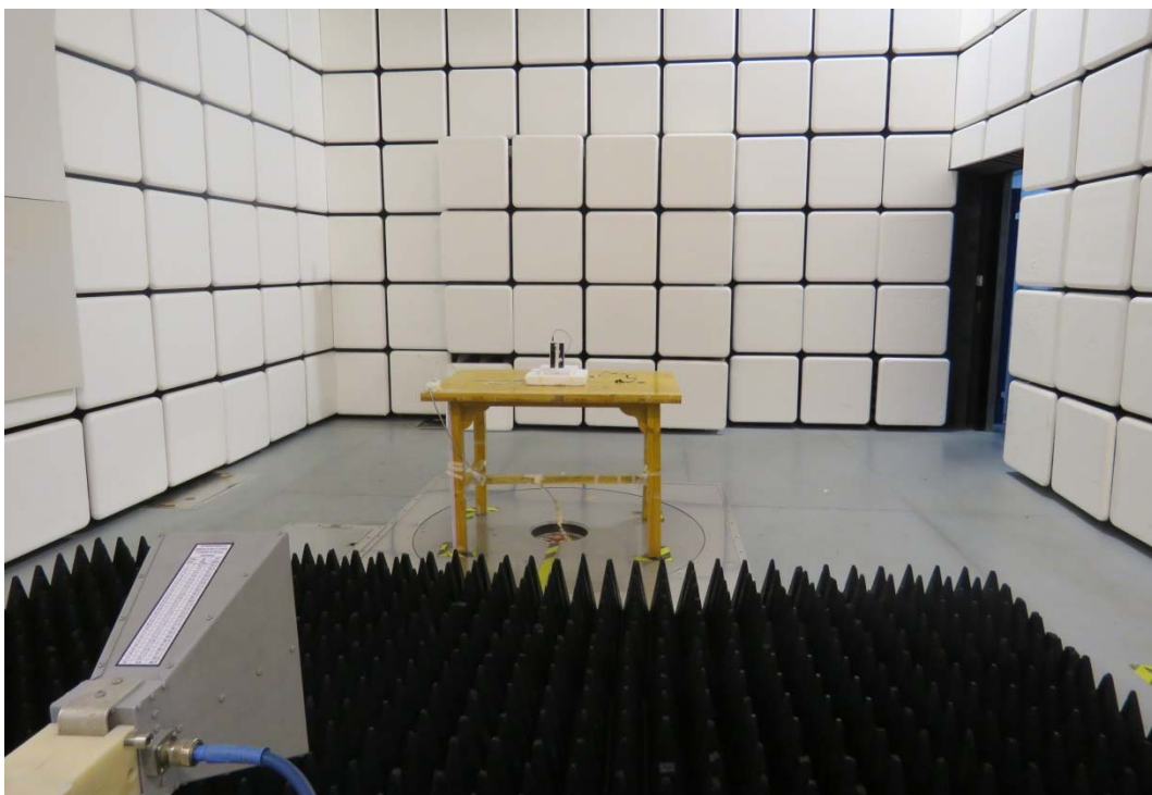
Picture 1: Radiated Spurious Emissions Test setup
