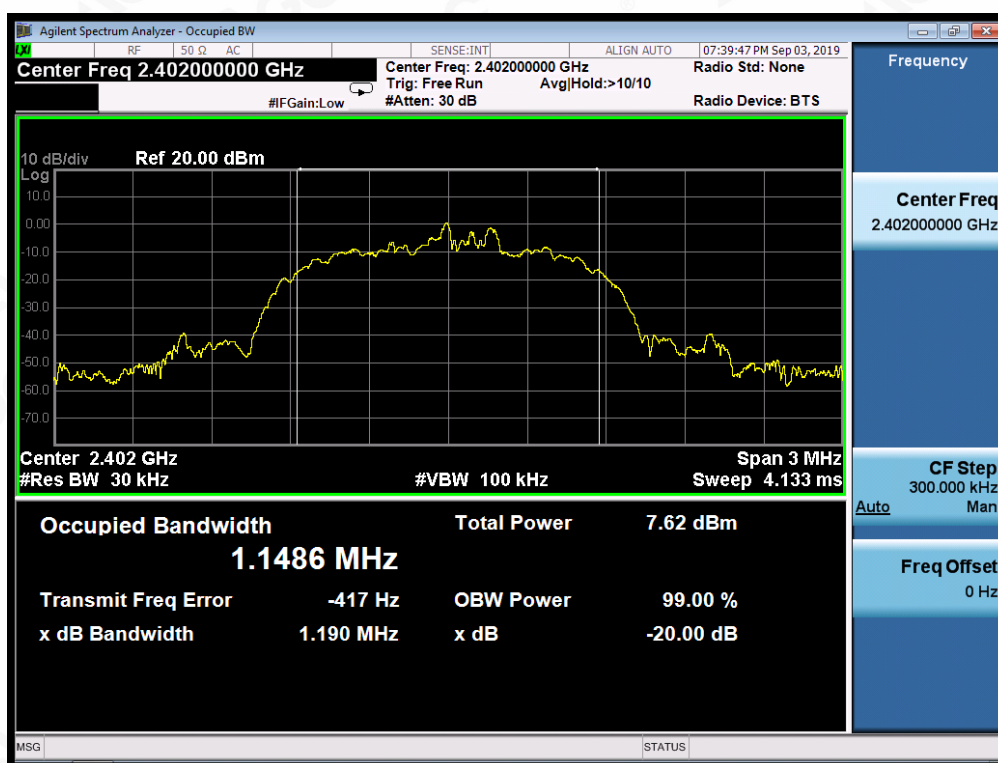
TEST PLOT OF BANDWIDTH FOR LOW CHANNEL
