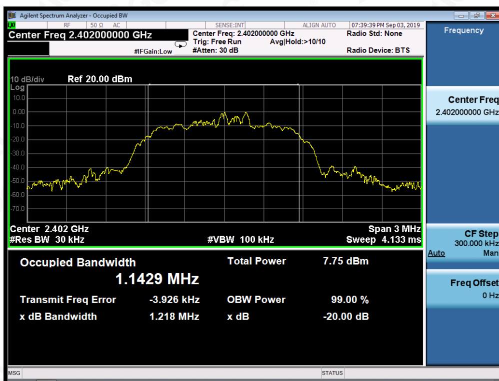
TEST PLOT OF BANDWIDTH FOR LOW CHANNEL
