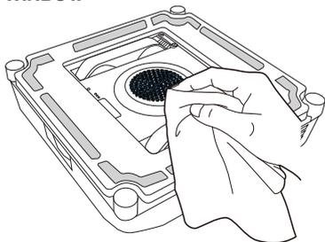
**Spherical Sensors:** Wipe clean with a dry cloth to maintain its sensitivity.
