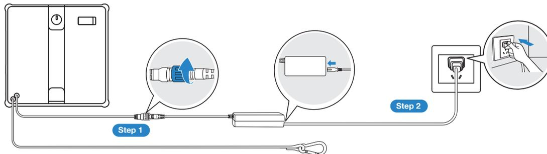
Connect correctly in the order shown above. Improper connection may cause charging abnormalities or damage to the battery.
