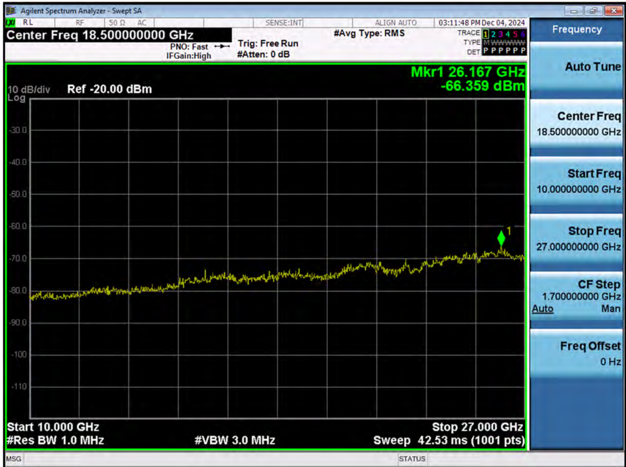
LTE B7_5 M_Conducted Spurious(10 G-26.5 G)_Low_QPSK_1RB
