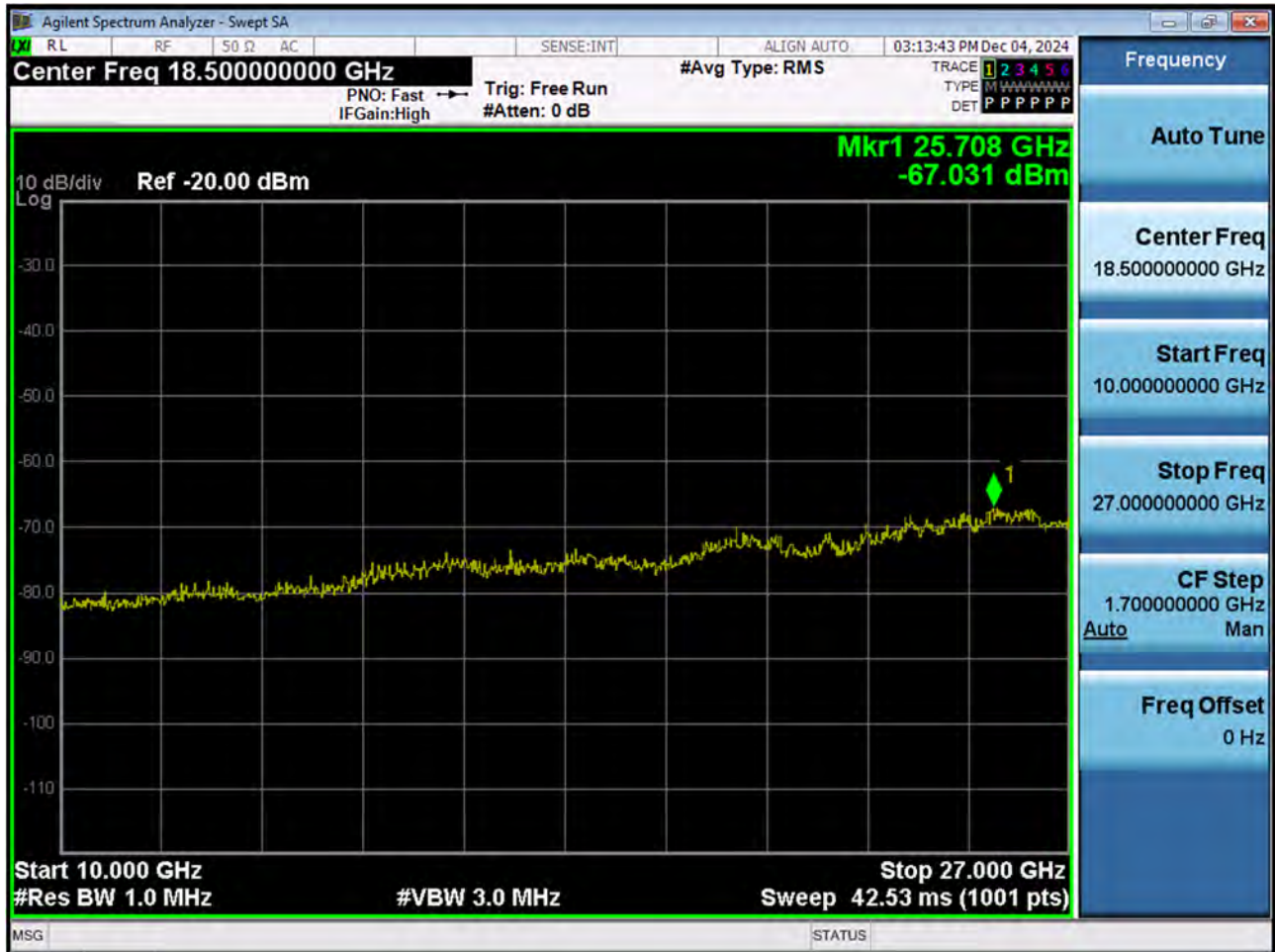
LTE B7_5 M_Conducted Spurious(10 G-26.5 G)_High_QPSK_1RB
