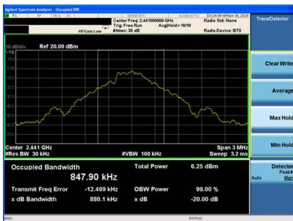
20dB Bandwidth plot on channel 78 (1Mbps)
