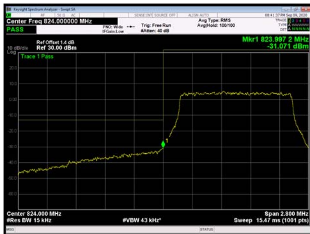
LTE Band 5 64QAM 3MHz CH-Low 1RB
