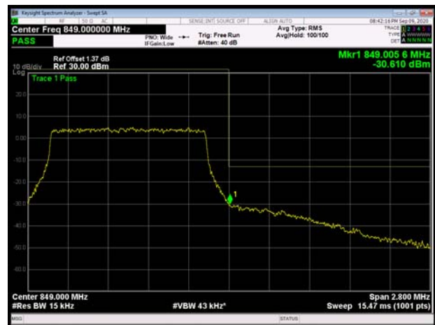
LTE Band 5 64QAM 3MHz CH-High 1RB
