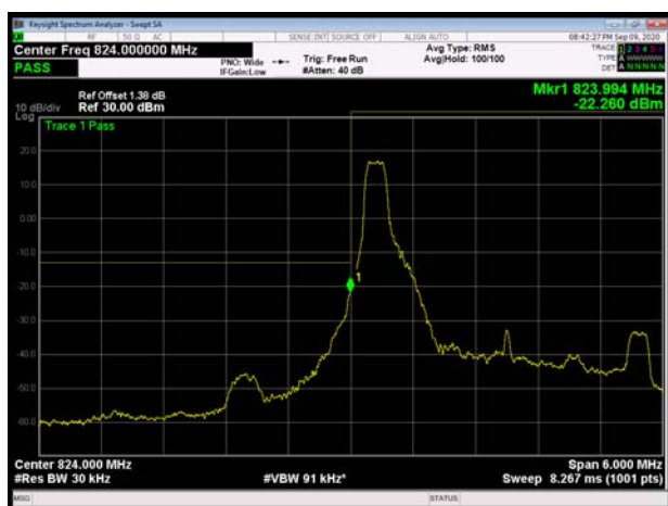
LTE Band 5 QPSK 3MHz CH-Low 100%RB
