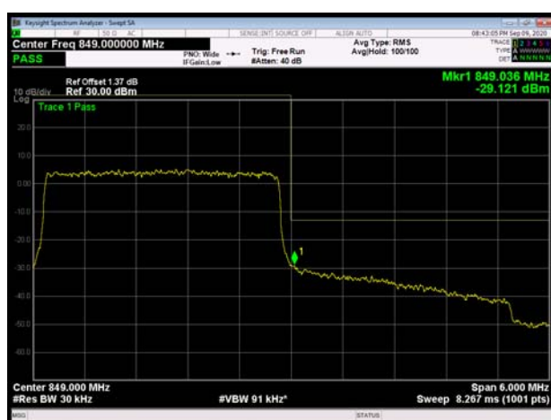
LTE Band 5 QPSK 5MHz CH-High 1RB
