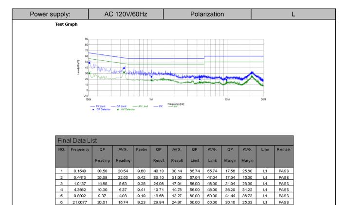
Note:1. Result (dB $\mu$ V) = Reading (dB $\mu$ V) + Factor (dB).
