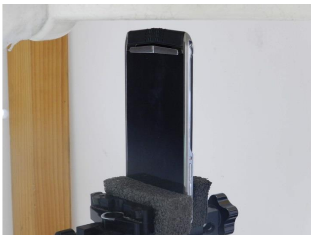
Bottom Side, Test Separation 1.0 cm
