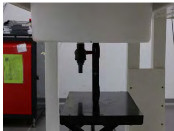
Fig.6 EUT Right side to flat phantom
