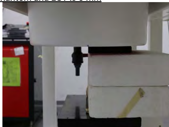
Fig.3 EUT Back side to flat phantom
