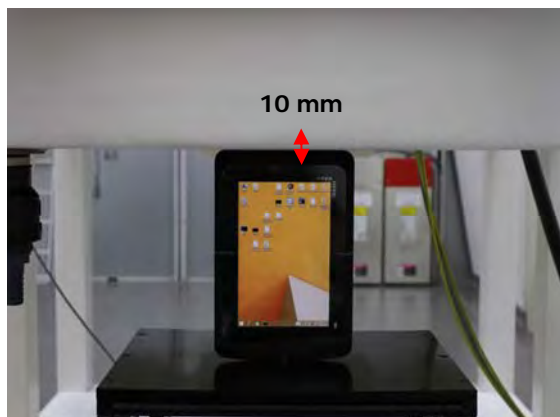
Fig.6 EUT Right side to flat phantom
