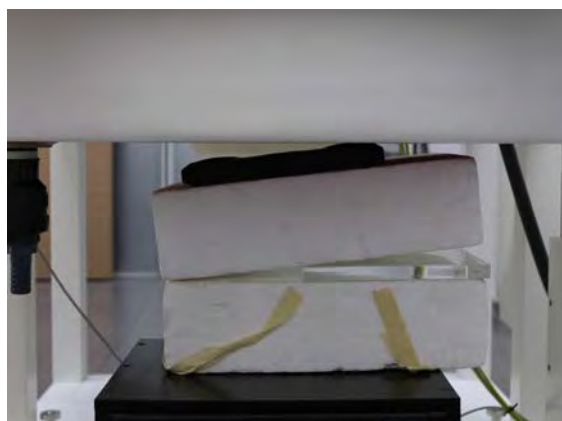
Fig.4 EUT Back side (Curve) to flat phantom
