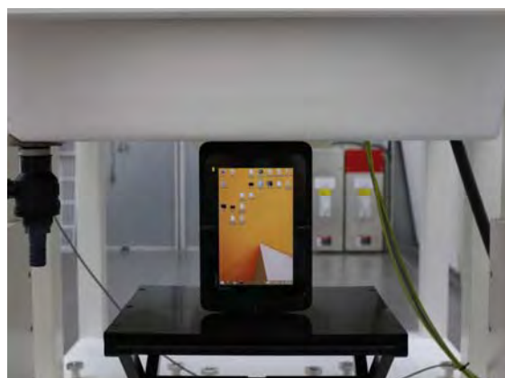
Fig.8 EUT Left side to flat phantom
