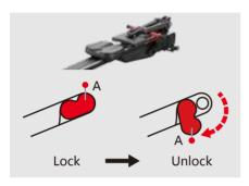
1 Locate the gas spring switch on the left and right sides of the center beam, turn the switch downwards to the UNLOCK position.
