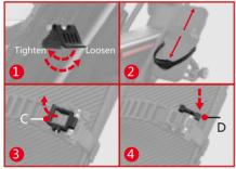
Ock buckle (part C) usage: Right pedal: Open the lock buckle upwards, hold and move it to left to quickly release the strap; the left pedal operates in the opposite direction.
