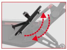
open the lock buckle, hold and move it to left (right) to quickly release the straps. Through the supportive gas spring at the bottom of the foot pedal, the motion posture of the foot can be adaptively raised or lowered.
