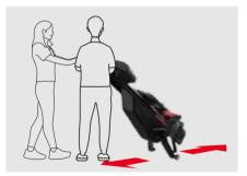
2 Use the transportation wheels on the front stabilizer to transport the rower to the desired location. Always hold the rear stabilizer during the entire movement.
