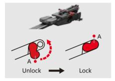
5 When the console is folded, remember to turn the switch upwards to the LOCK position.
