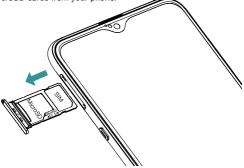
To eject SIM or MicroSD cards, insert your SIM eject pin into the small hole next to the card tray.
